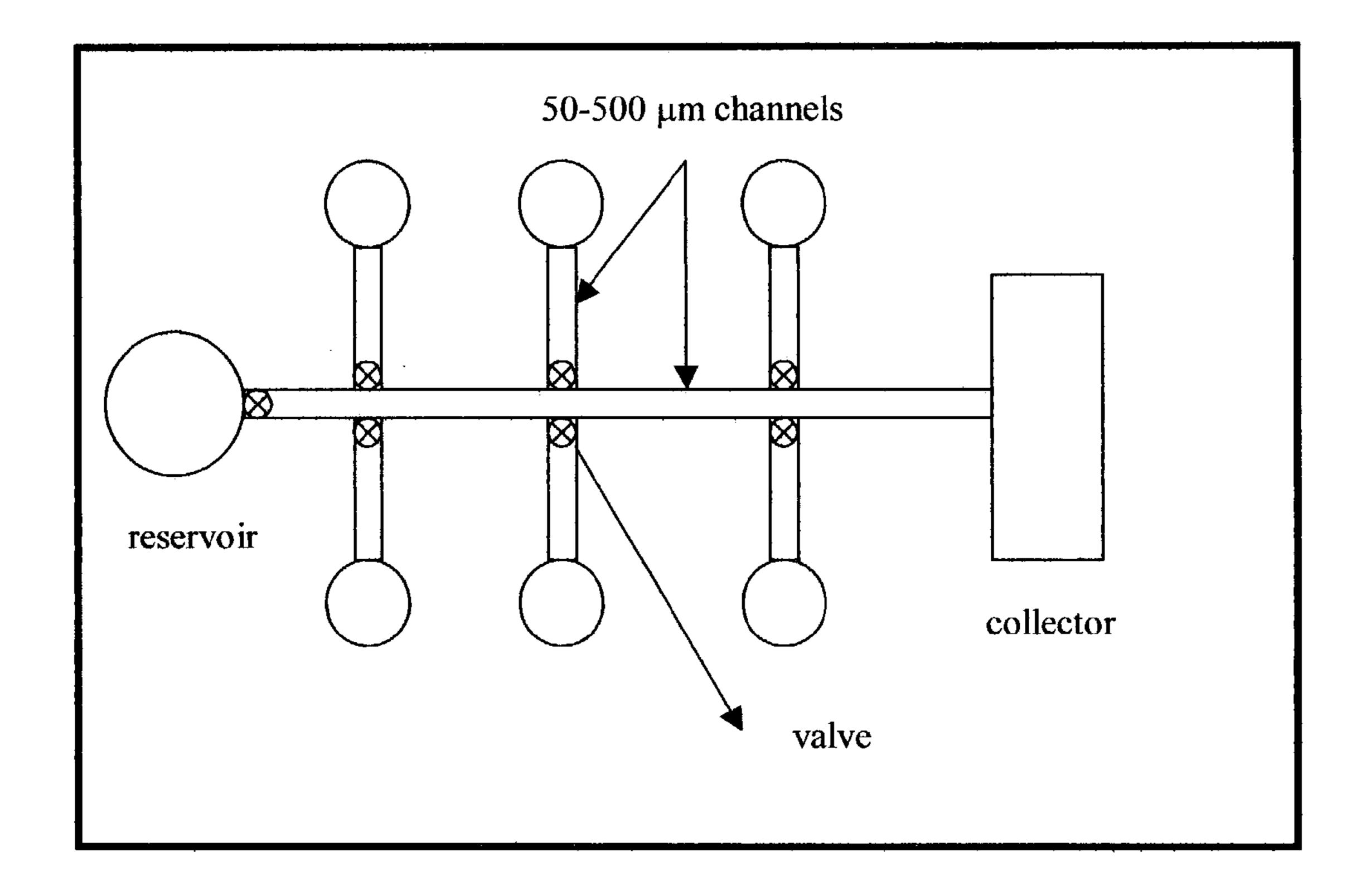
Figure 3 (a) Advanced Microfluidic Plate
