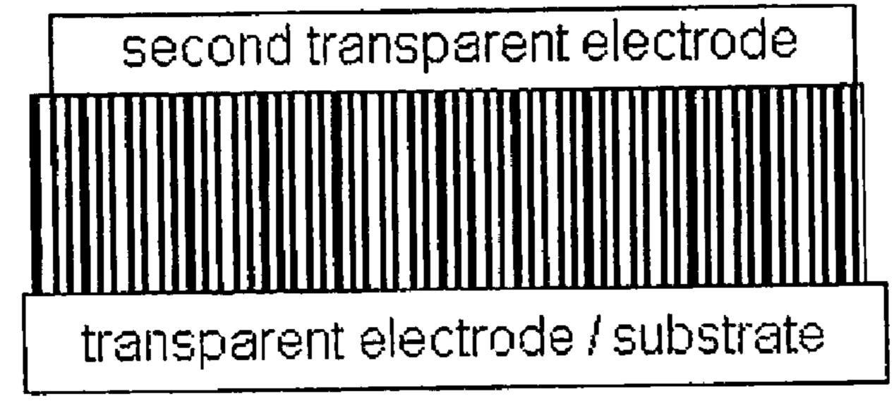
first transparent electrode/ porous template/ conducting polymer/ , electrolyte 1
