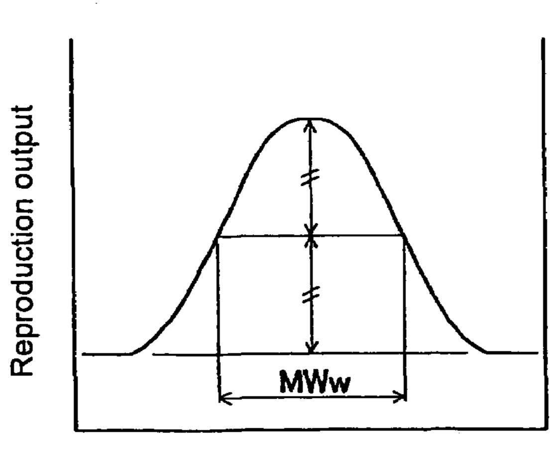
Position of reproducing head in track width direction
