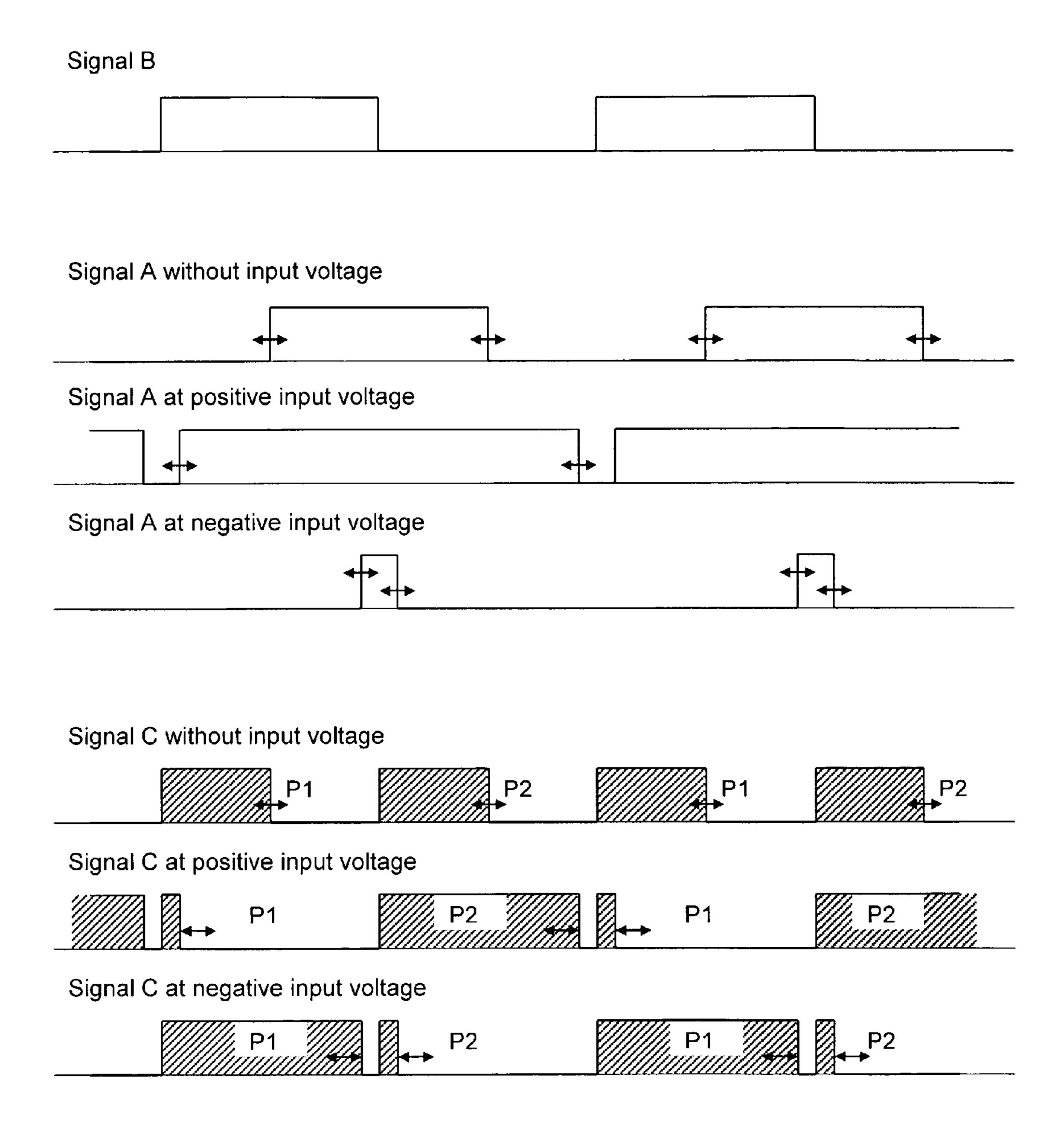
Fig. 3: Measurement of pulse lenght using a delay line
