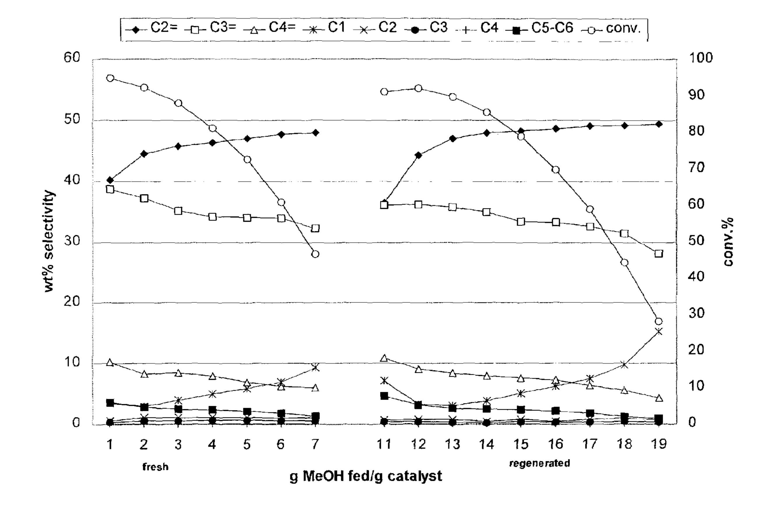
Figure 4. Conversion and selectivity for fresh (left) and regenerated (right) SAPO-34 modified with ZnMe<sub>2</sub> (Example 24, Sample B)
