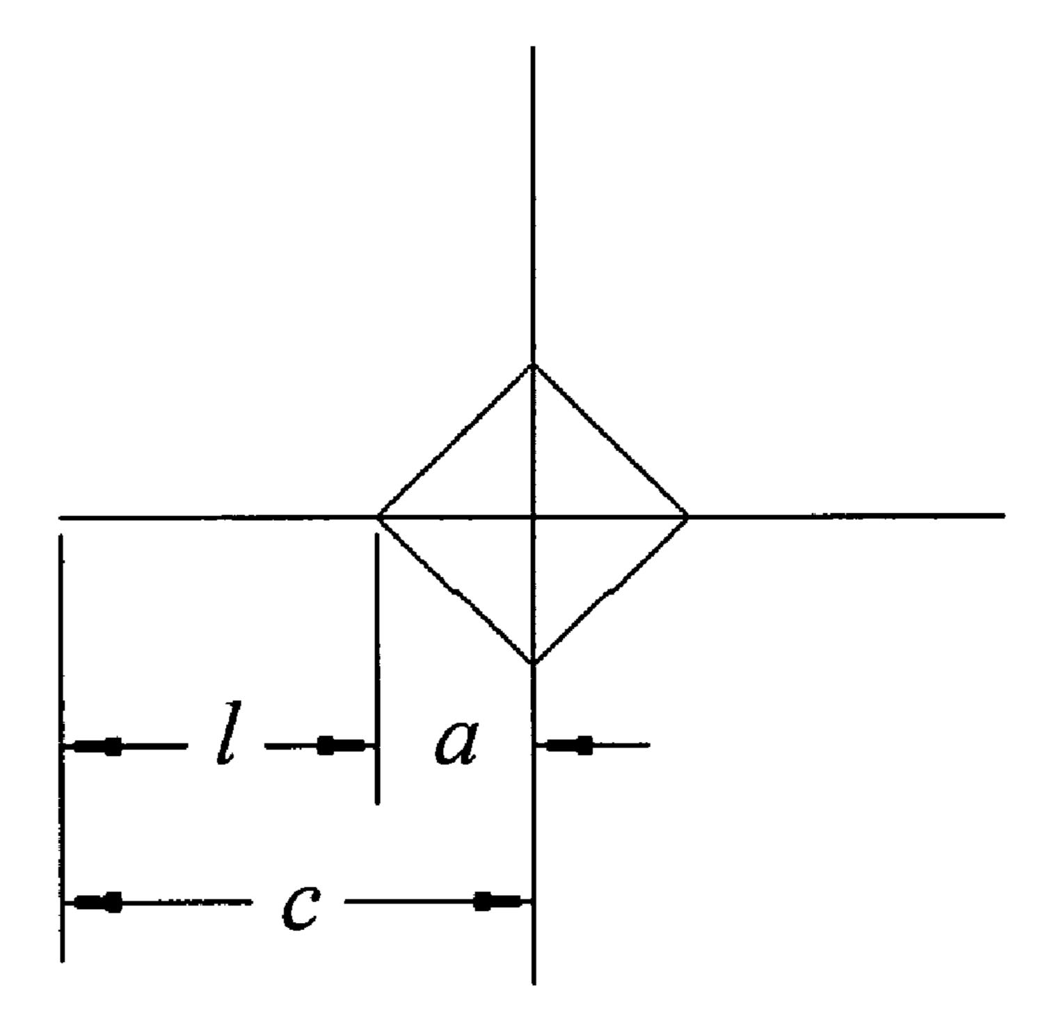
Figure 1. Plane view of Vickers indentation with radial cracks.
