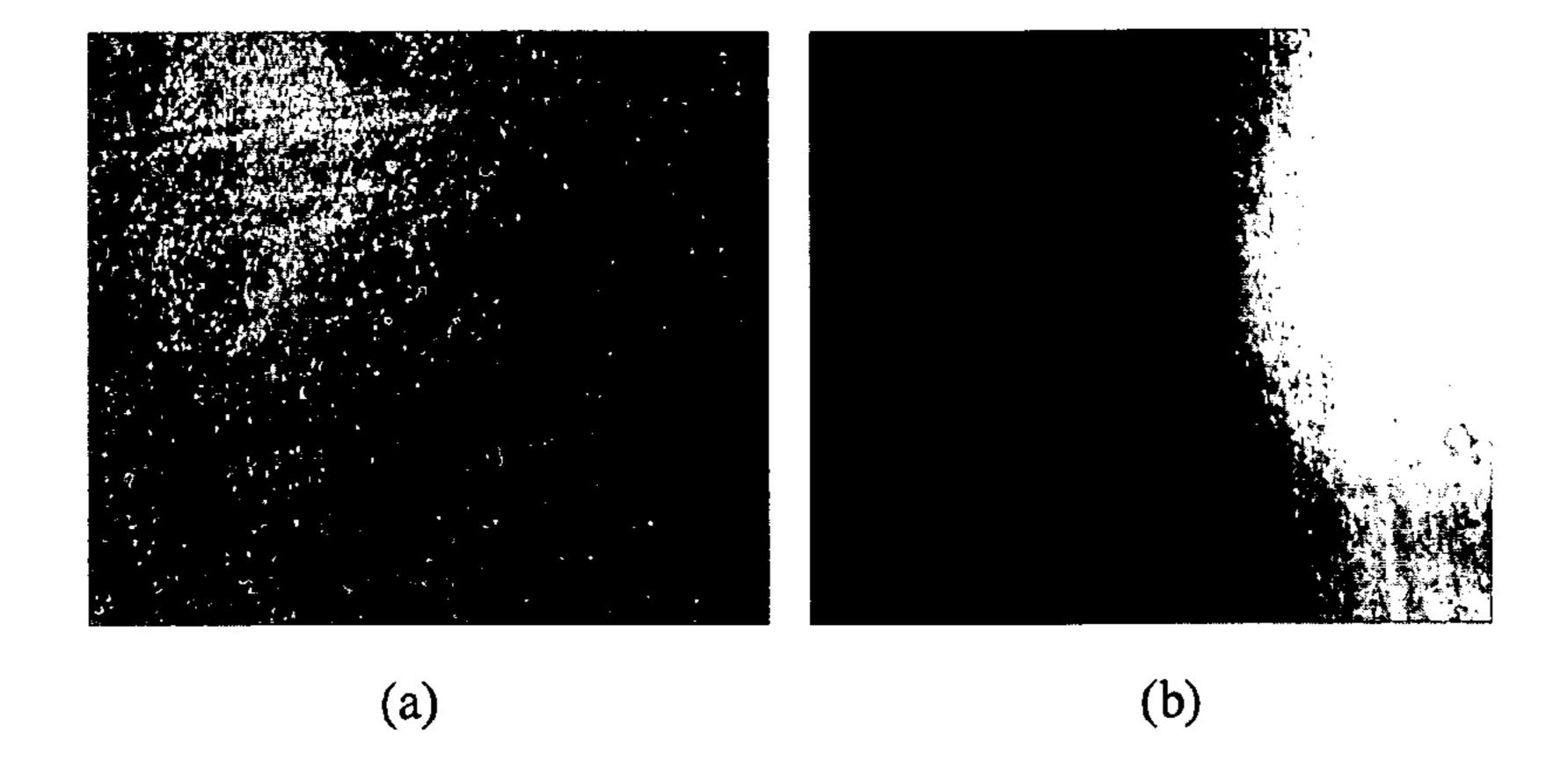
Figure 6. Vickers indentation on an 8YSZ specimen at about 300x magnification. (a) without shadow, (b) with shadow introduced from left by the frame edge.
