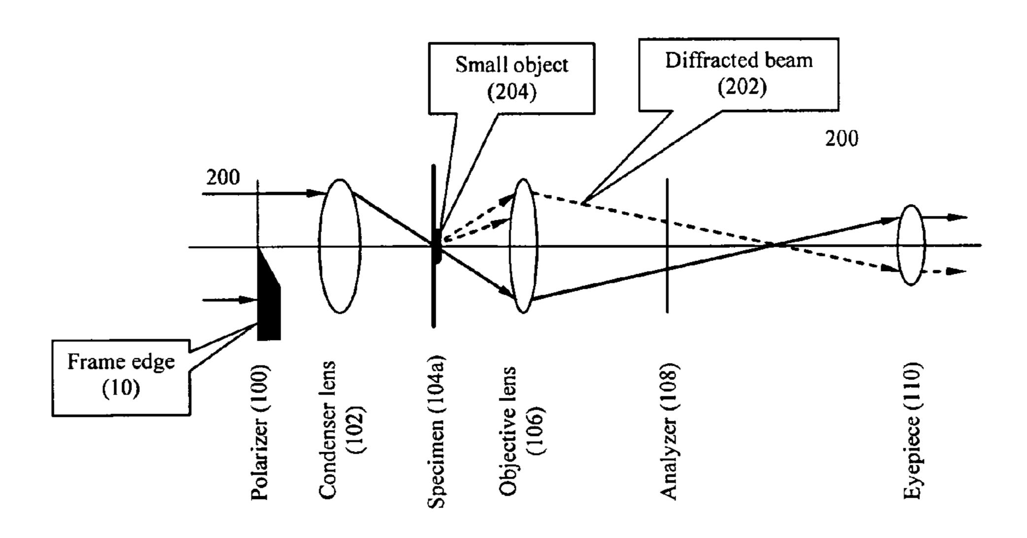
Figure 4. A close-up view of specimen stage and eyepiece of the modified microscope. The solid lines represent unobstructed beams, and the dashed lines are diffracted beams from the object (crack line).
