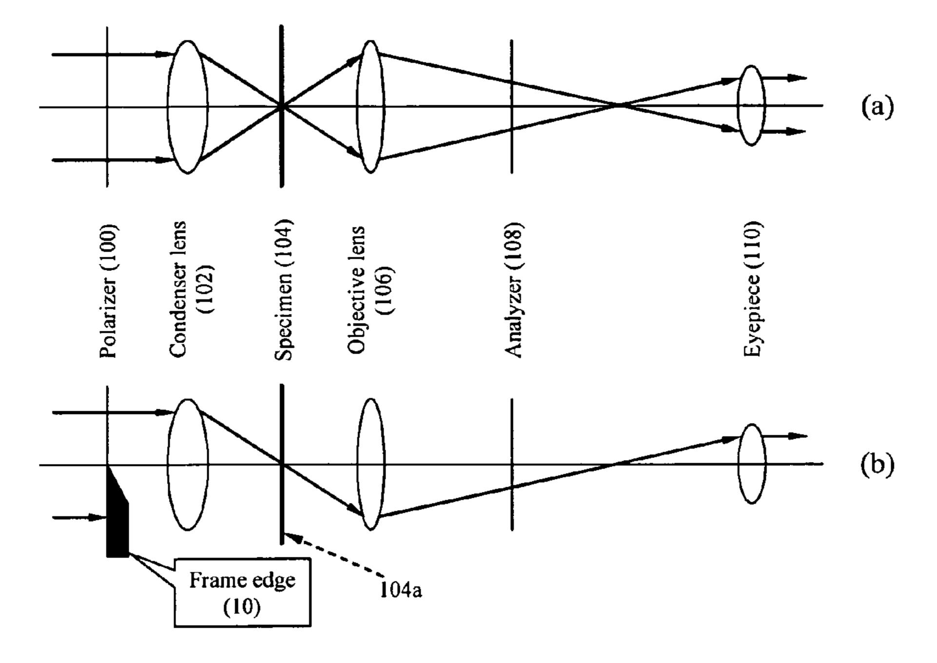
Figure 3. (a) Conventional polarizing microscope; (b) modified microscope with a frame edge positioned at the middle of the field of view. The optical systems are simplified and the illumination optical paths (Condenser lenses) are unfolded schematically for clarity.
