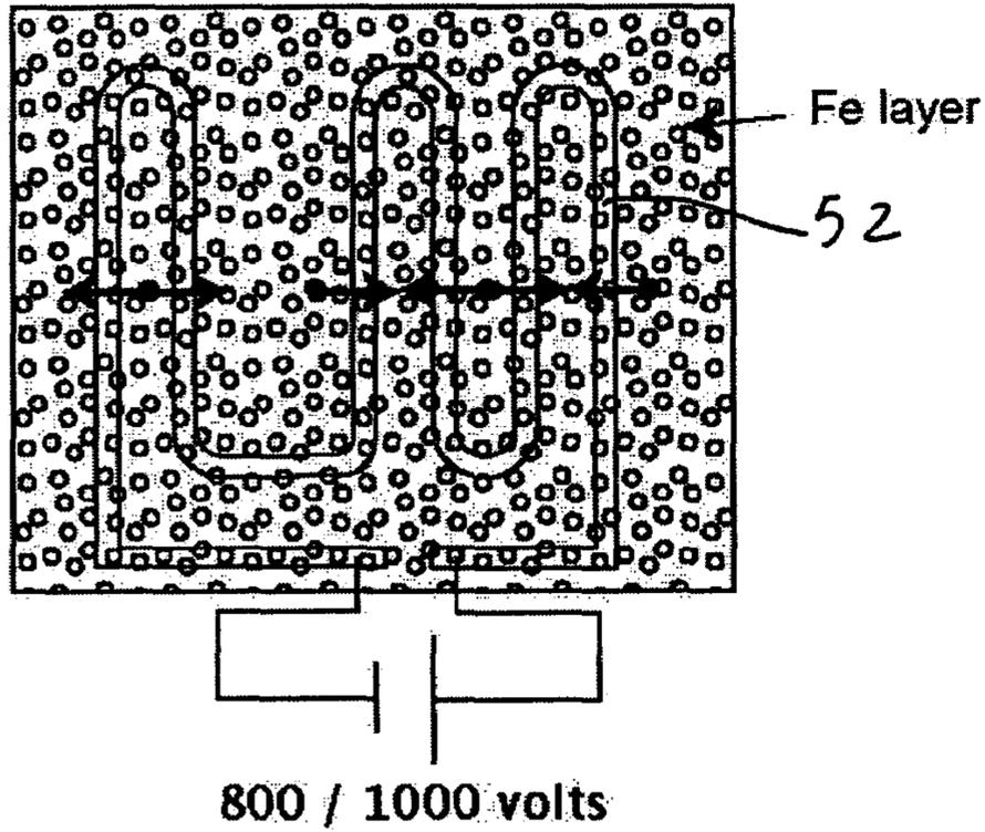
Fig 18: Simple coil configuration to direct a vehicle:
