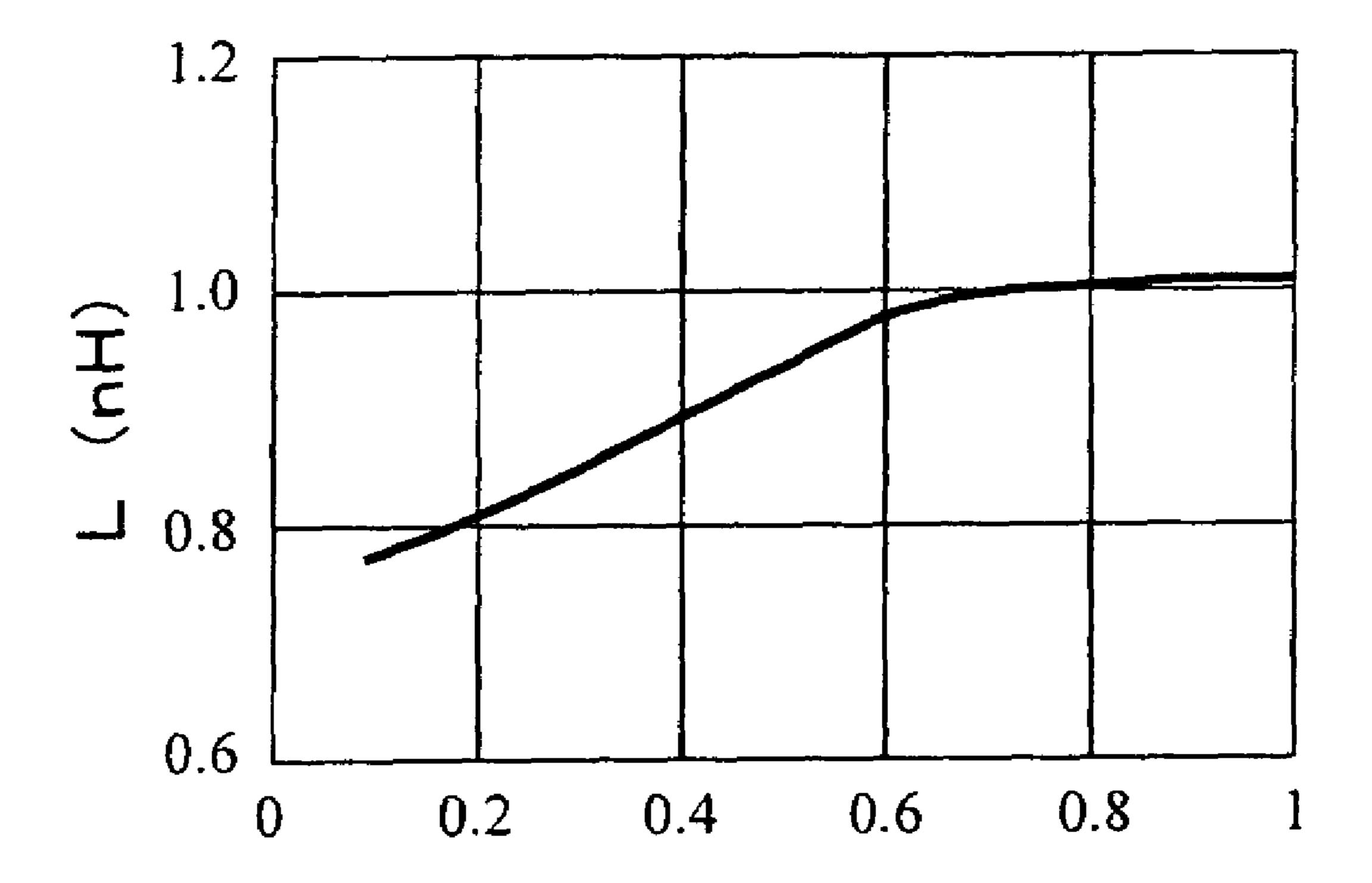
Distance between metal shielding cap and chip inductor (mm)
