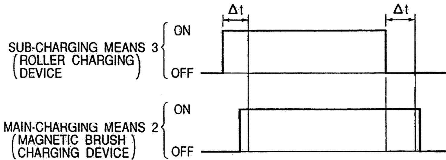
$\Delta t$ : TIME REQUIRED FOR PHOTOSENSITIVE DRUM SURFACE, WHICH HAD BEEN IN CHARGING AREA "b" OF SUB-CHARGING MEANS 3, REACHING CHARGING AREA "a" OF MAIN-CHARGING MEANS 2
