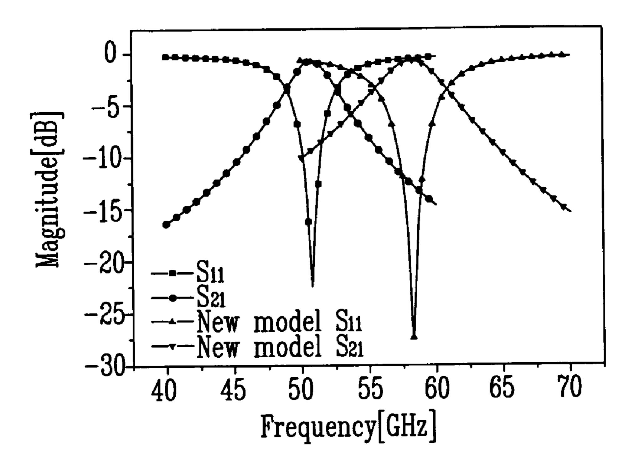
FIG.8 60 GHz Bandpass Filter
