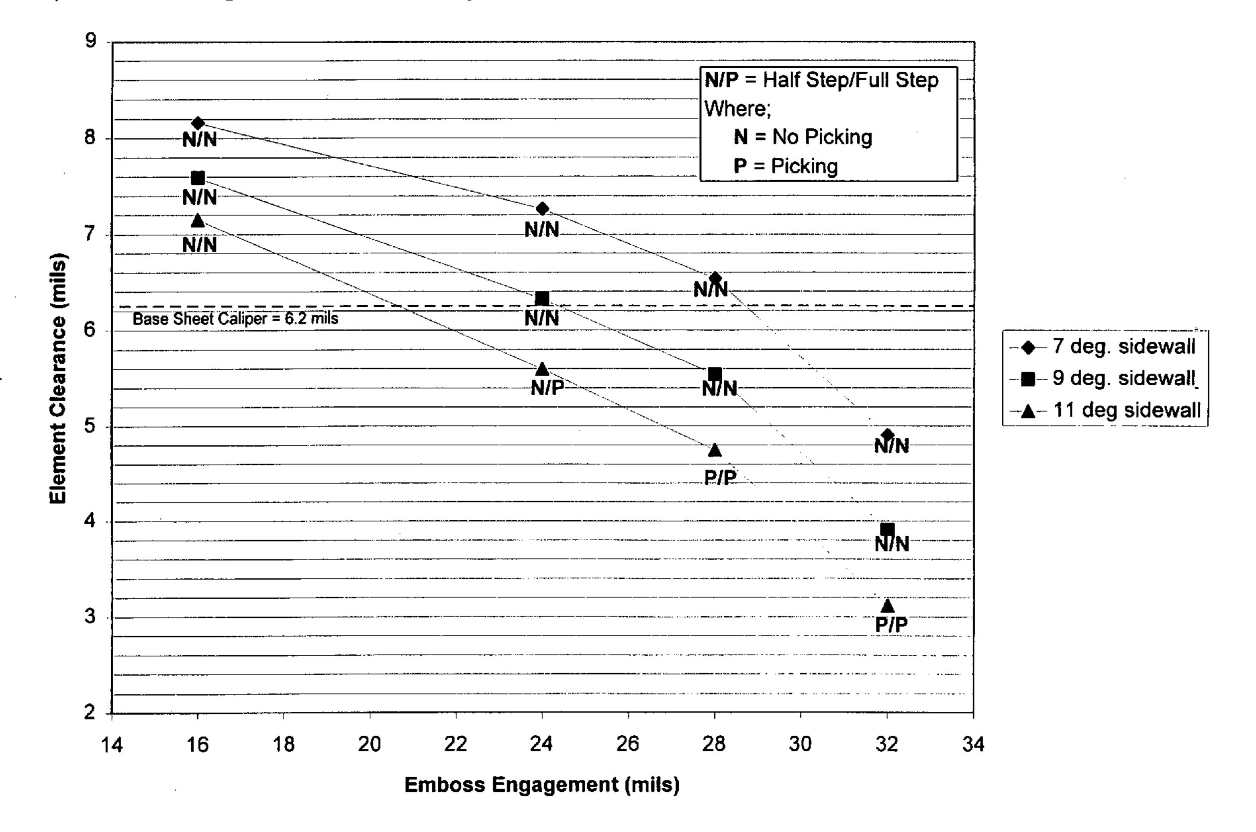
FIG. 19 shows that for this particular trial using embossing rolls having a 45 mil element height, picking did not occur at any of the sidewall angles. However, as shown in FIG. 20, when the embossing rolls having a 42.5 mil element height were run, fiber picking was observed on the 11° 5 sidewall angle elements at the higher embossing engagements, i.e., 24, 28, and 32 mils. No fiber picking was encountered with elements having sidewall angles of 7° or 9°.
