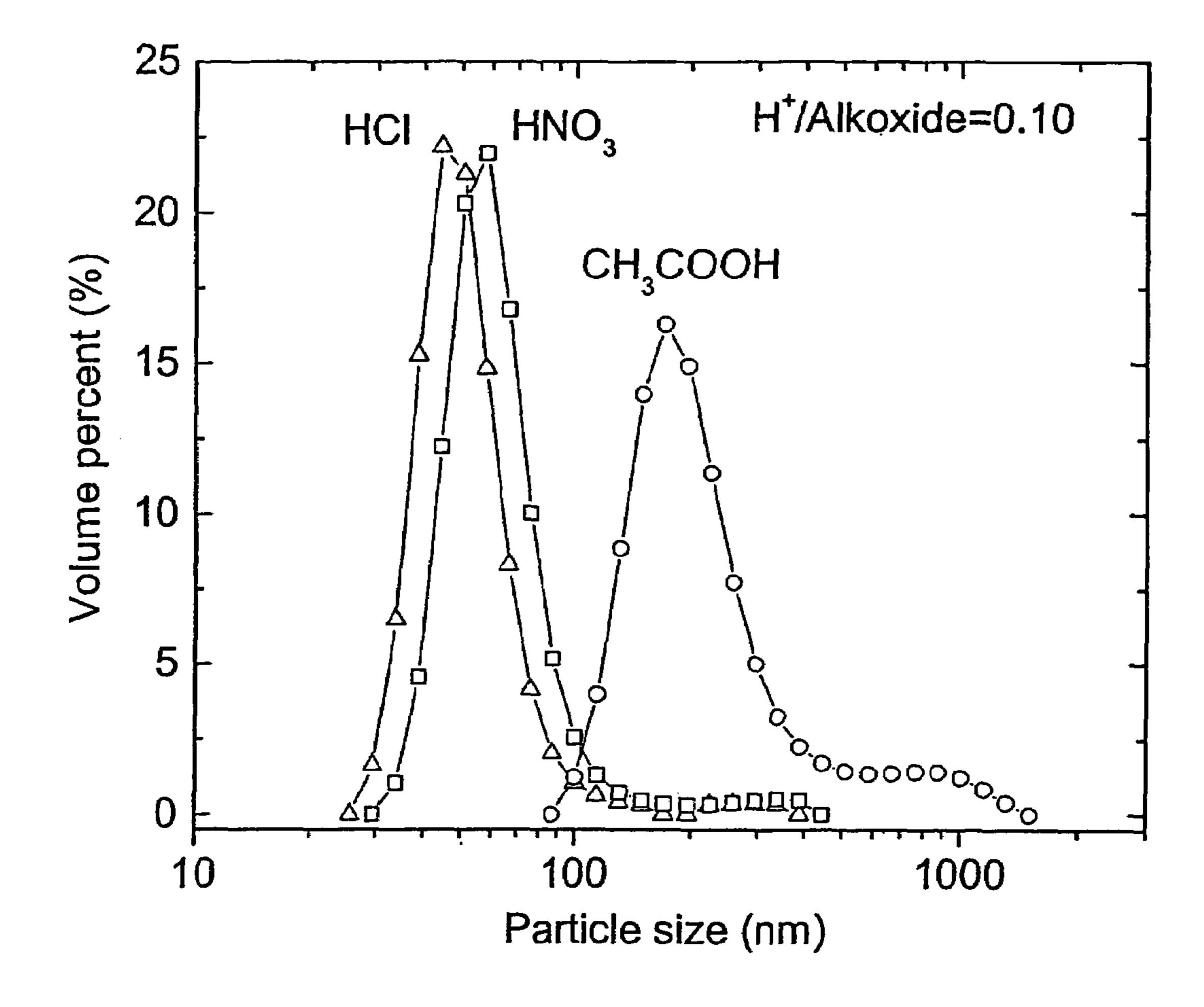
Figure 3. Particle Size Distributions of Boehmite Sols Peptized with Acetic Acid. Molar ratio of H<sup>+</sup>/Alkoxide are indicted.
