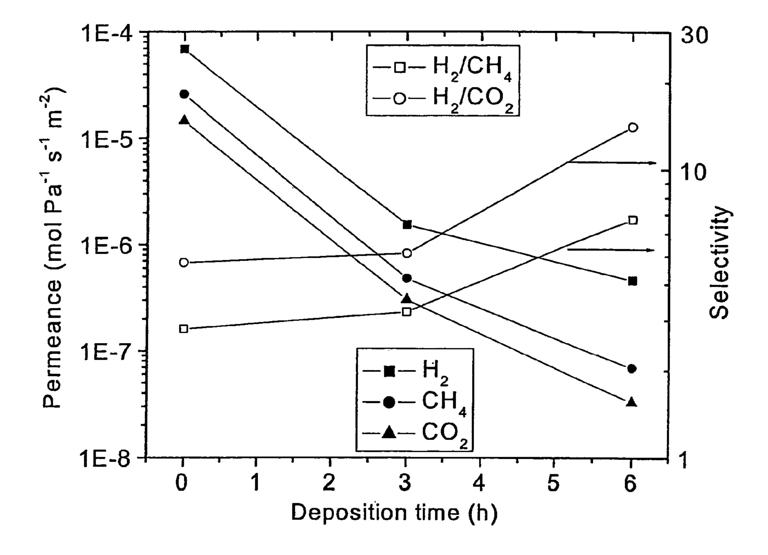
Figure 9. Permeation Properties at 873 K of a Graded Four-Layer Silica/Alumina Membrane.
