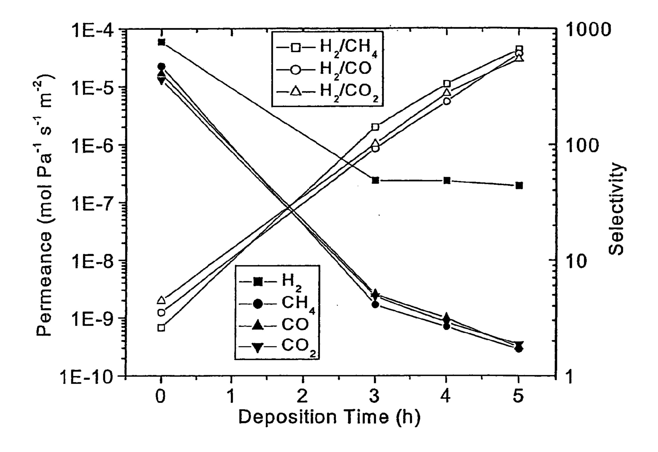
Figure 10. Permeation Properties at 873 K of a Graded Five-Laver Silica/Alumina Membrane.
