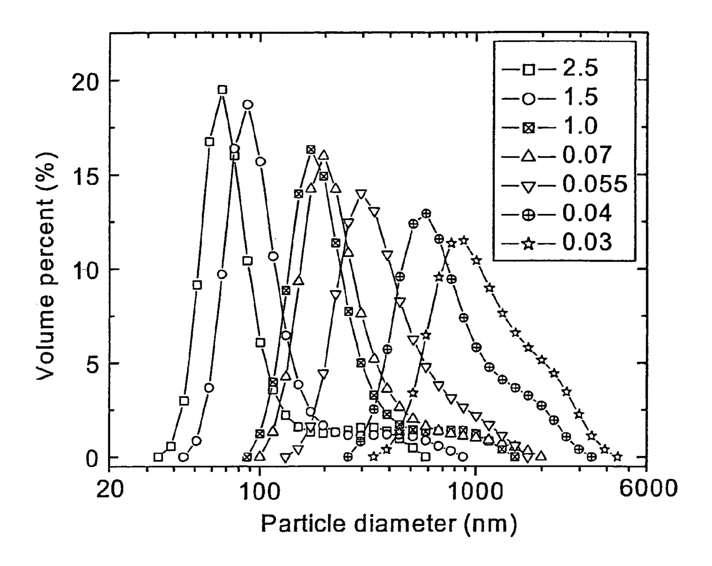
Figure 4. Particle Size Distributions of Boehmite Sols Hydrolyzed for Different Times
