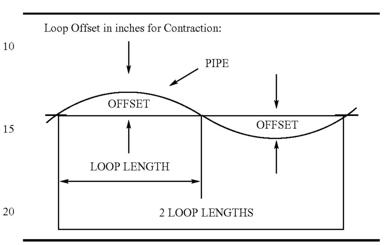
Maximum Temperature Variation, ° F., Between Time of Solvent Welding and Final Use 60° 70°  $80^{\circ}$ 90° 100° 10° 20° 30° 40° 50° Loop Length LOOP OFFSET 20 Feet 7" 9" 11" 13" 16" 50 Feet 13" 18" 22" 26" 100 Feet
