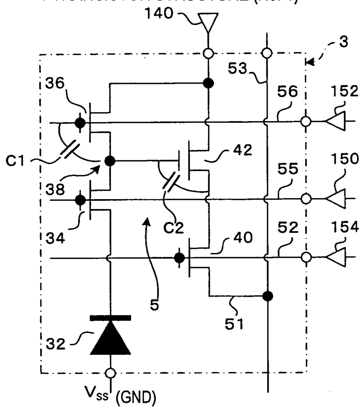
4-TRANSISTOR STRUCTURE (No. 2)
