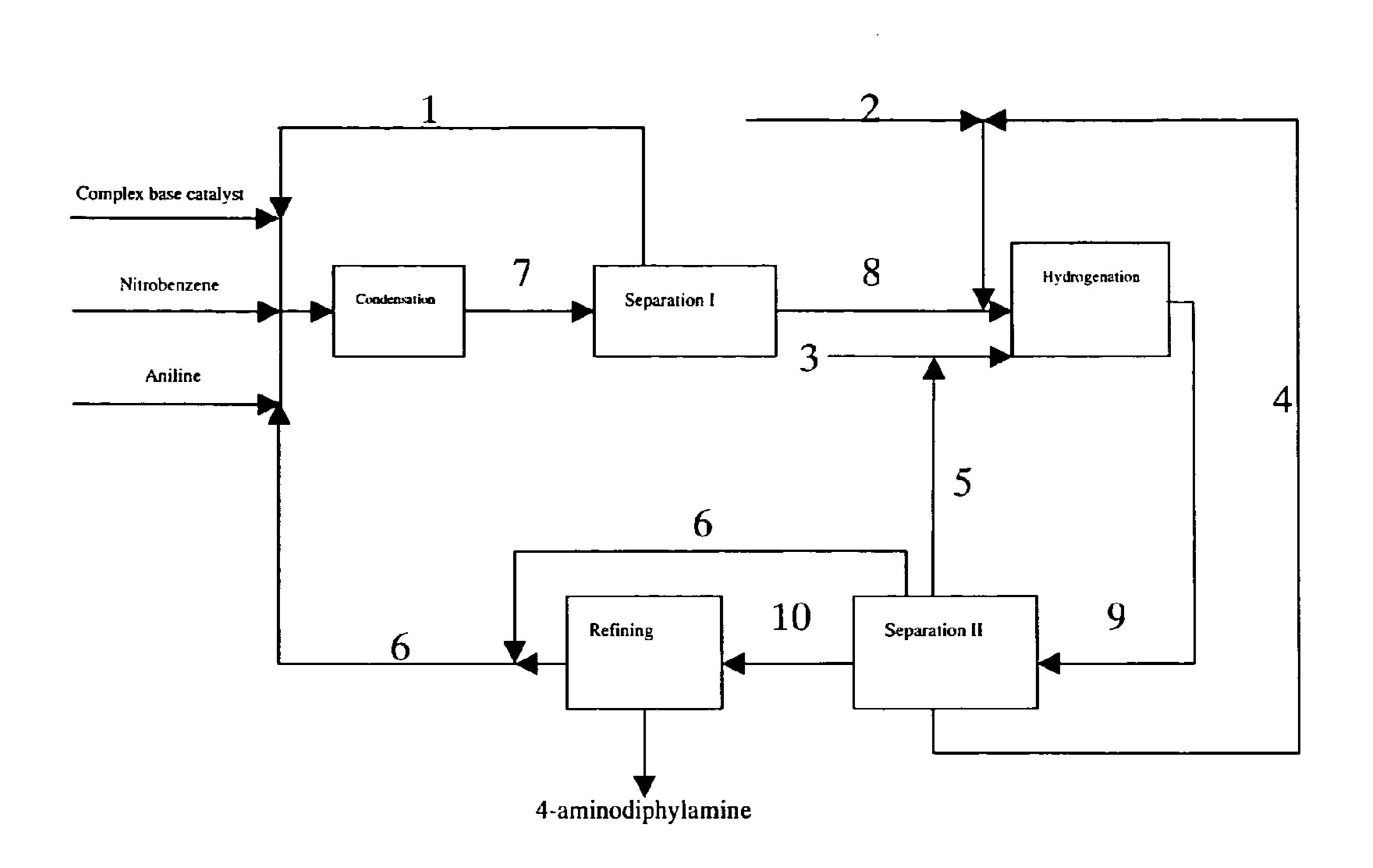
Figure 1. A flow diagram of the process for preparing 4-aminodiphylamine
