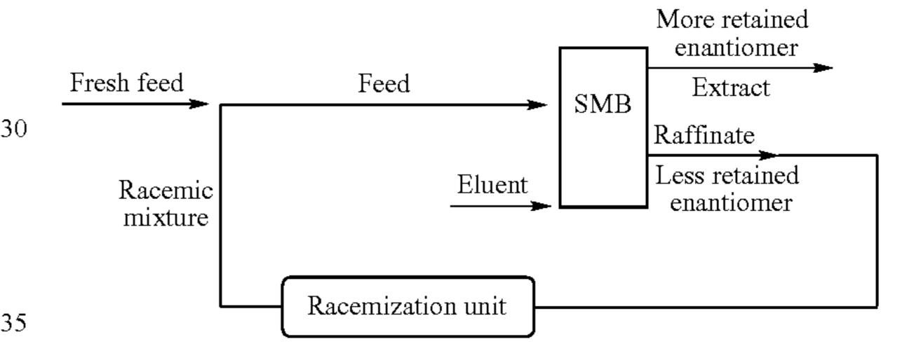
The more retained enantiomer (+) may be recovered at the required optical purity (95–99.9%) in the extract stream whereas the less retained enantiomer (-) may be collected in the raffinate stream. It may be possible to recycle the stream enriched in the undesired enantiomer through a racemization unit, which would decrease the necessary amount of new racemic feed required.
