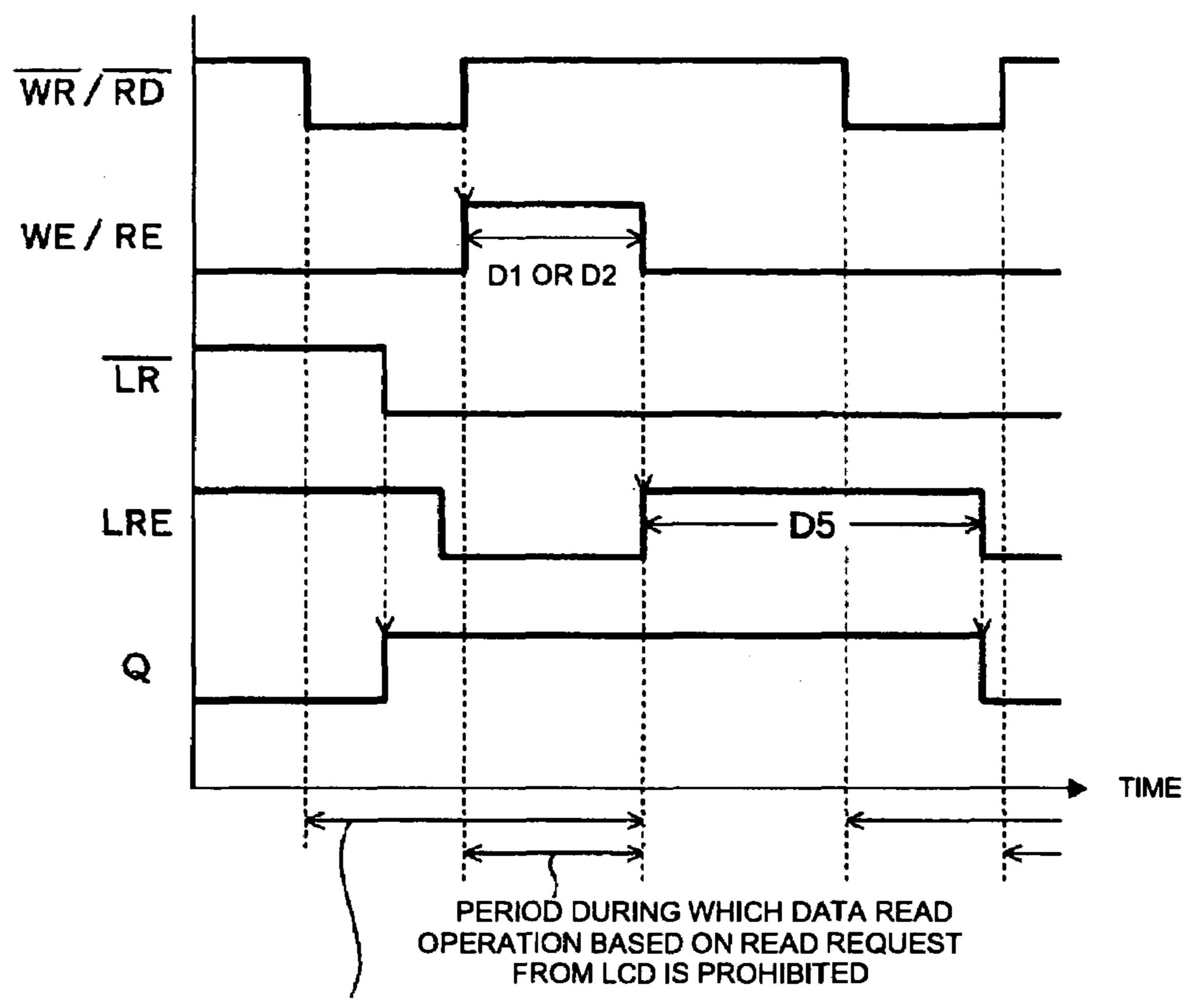
PERIOD DURING WHICH START OF DATA READ OPERATION BASED ON READ REQUEST FROM LCD IS PROHIBITED
