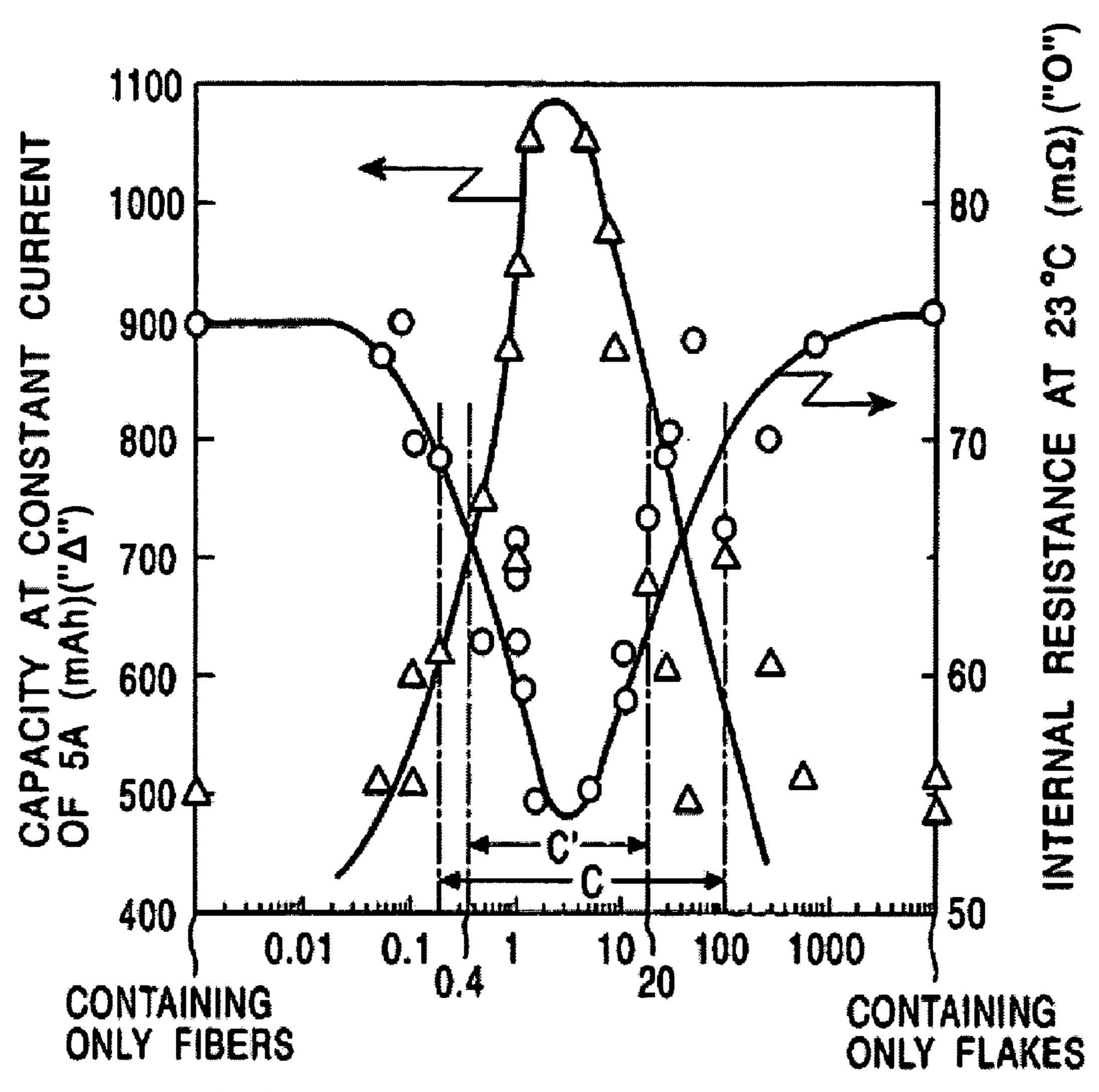
RATIO BY WEIGHT OF CARBON FLAKES KS-15 TO CARBON FIBERS VGCF
