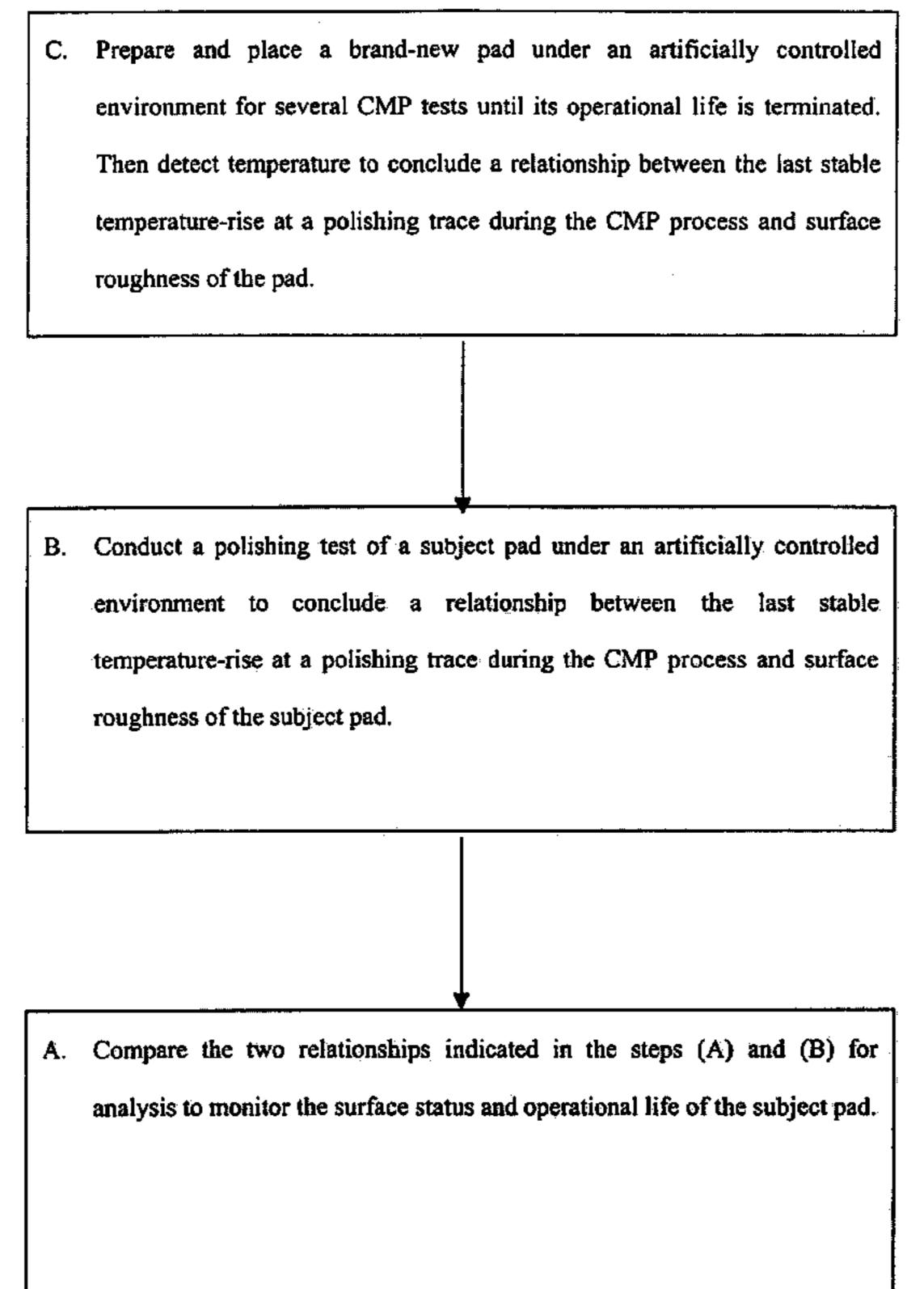
C. Prepare and place a brand-new pad under an artificially controlled environment for several CMP tests until its operational life is terminated. Then detect temperature to conclude a relationship between the last stable temperature-rise at a polishing trace during the CMP process and surface roughness of the pad.
