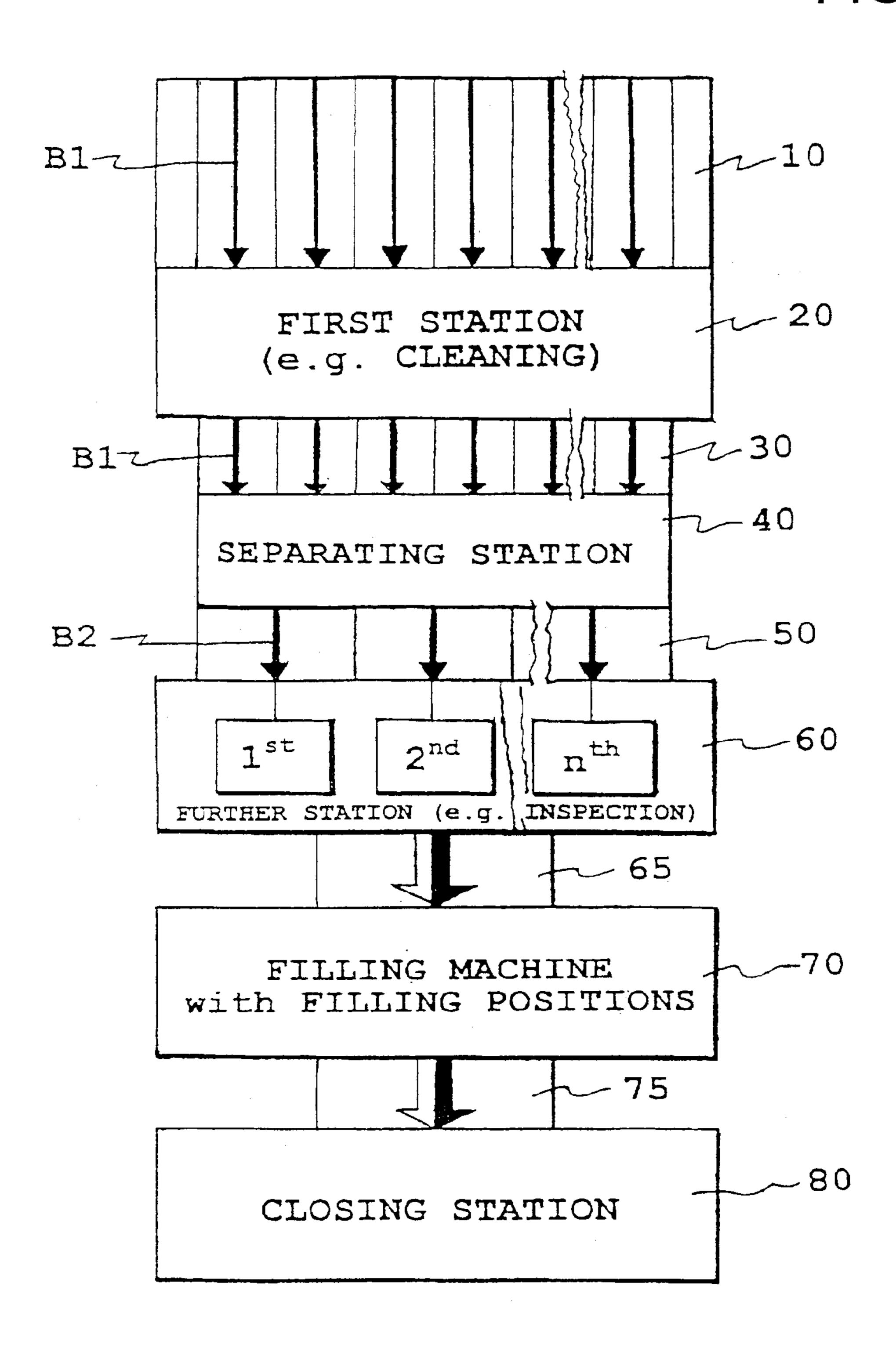
BEVERAGE BOTTLING PLANT FOR FILLING BEVERAGE BOTTLES OR OTHER BEVERAGE CONTAINERS WITH A LIQUID BEVERAGE FILLING MATERIAL AND AN ARRANGEMENT FOR DIVIDING AND SEPARATING OF A STREAM OF BEVERAGE **BOTTLES OR OTHER BEVERAGE** CONTAINERS
