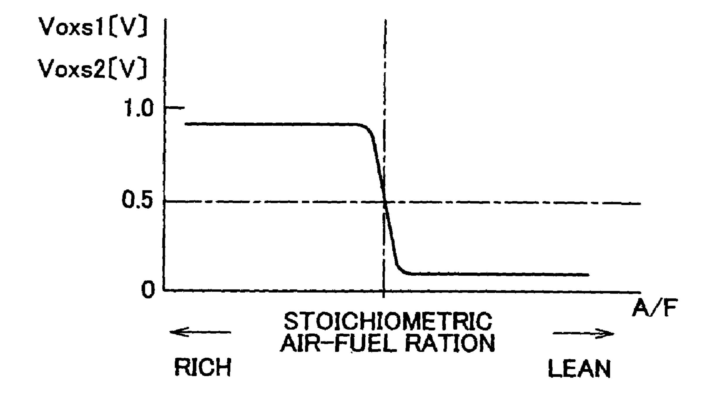
Mode=1 0 0 STOICHIOMETRIC AIR-FUEL RATIO (C)OXYGEN STORAGE OF-FIRST CATALYST (E)OXYGEN STOI OF SECOND CAT
