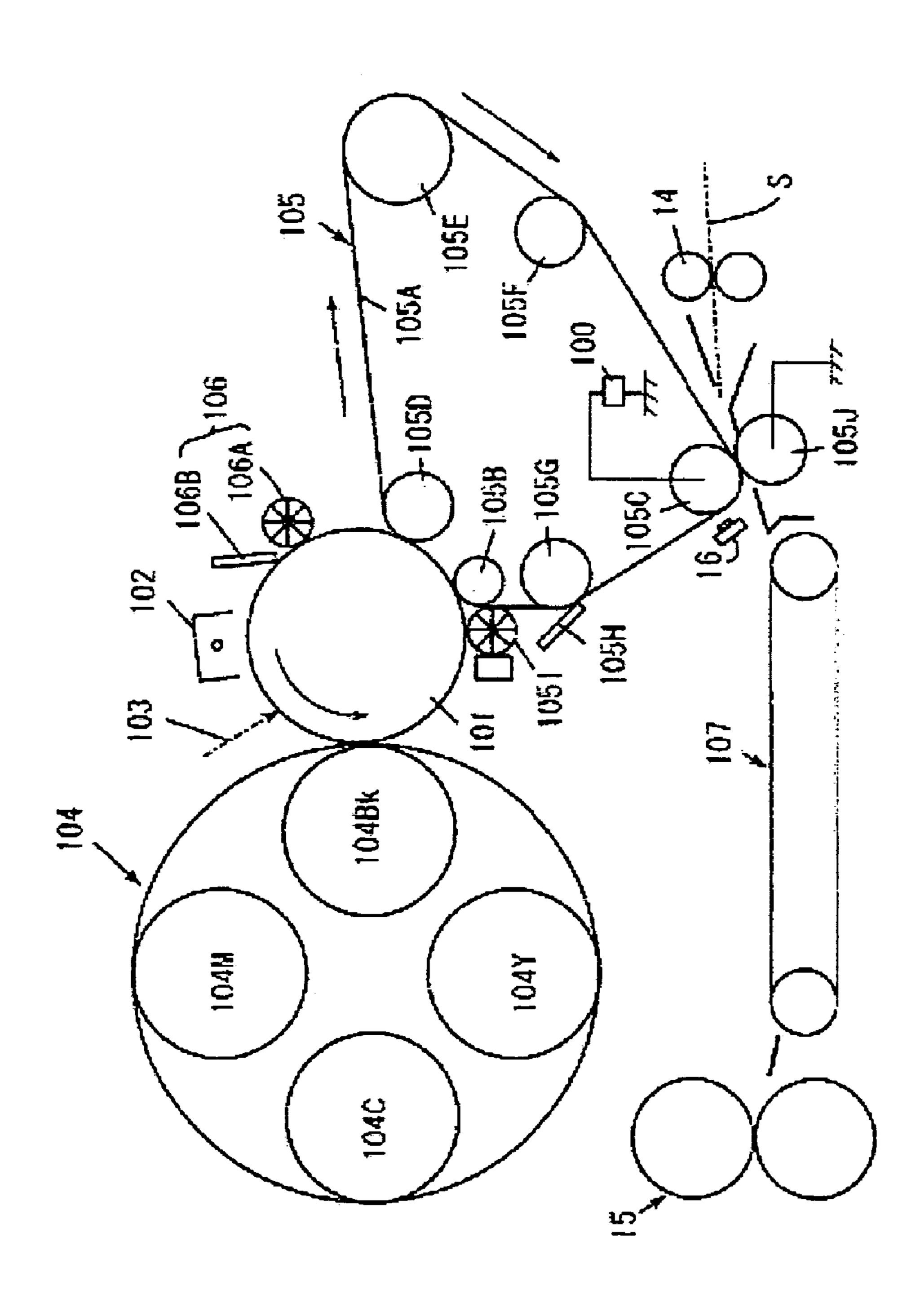
METHOD AND APPARATUS FOR IMAGE FORMING CAPABLE OF EFFECTIVELY PREVENTING TONER ADHESION ON A DENSITY SENSOR BY GENERATING AN ELECTRIC FIELD ACCORDING TO A VISIBLE IMAGE
