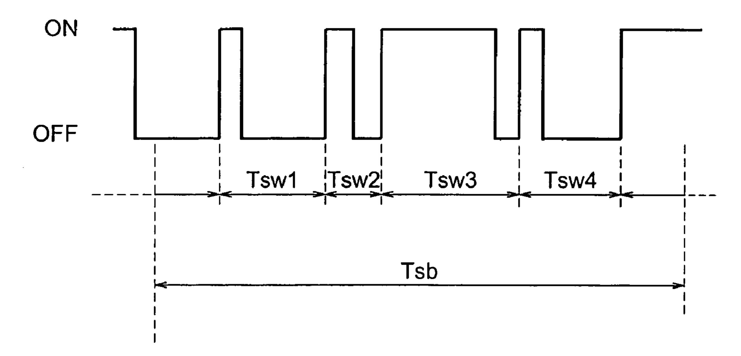
Tsw 1 to Tsw4: FIELD SWITCH CYCLE TSb: SAMPLING CYCLE
