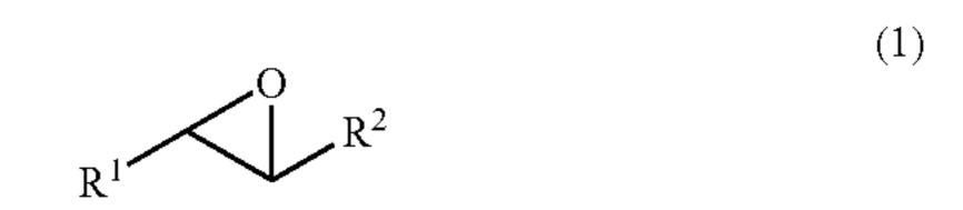
wherein R<sup>1</sup> and R<sup>2</sup> are the same or different, an organic group not containing aldehyde group or ketone group therein or hydrogen atom, provided that both R<sup>1</sup> and R<sup>2</sup> are not simultaneously hydrogen atom.
