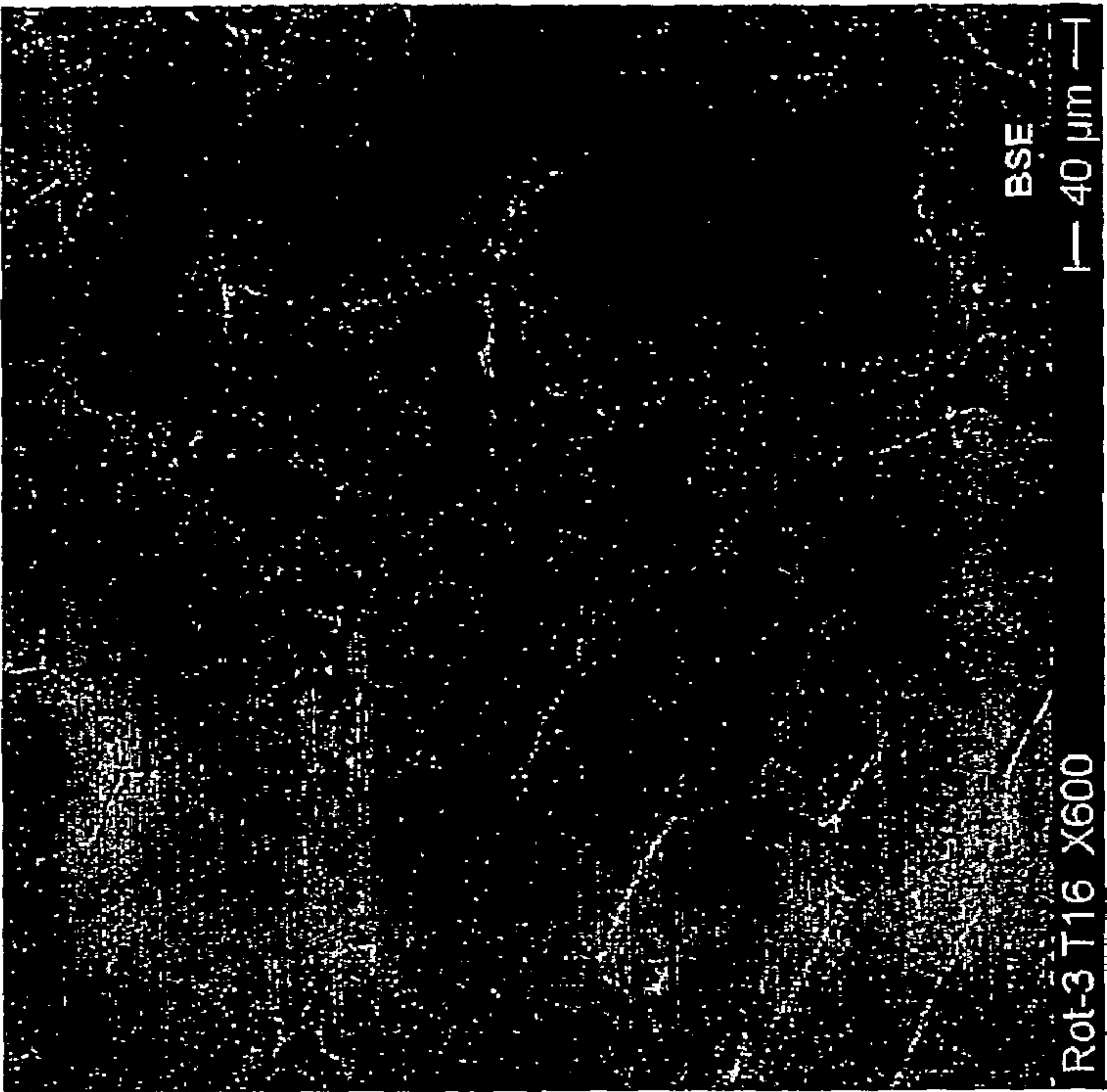
High Temperature Sintered for 150 min. at 1300° C
