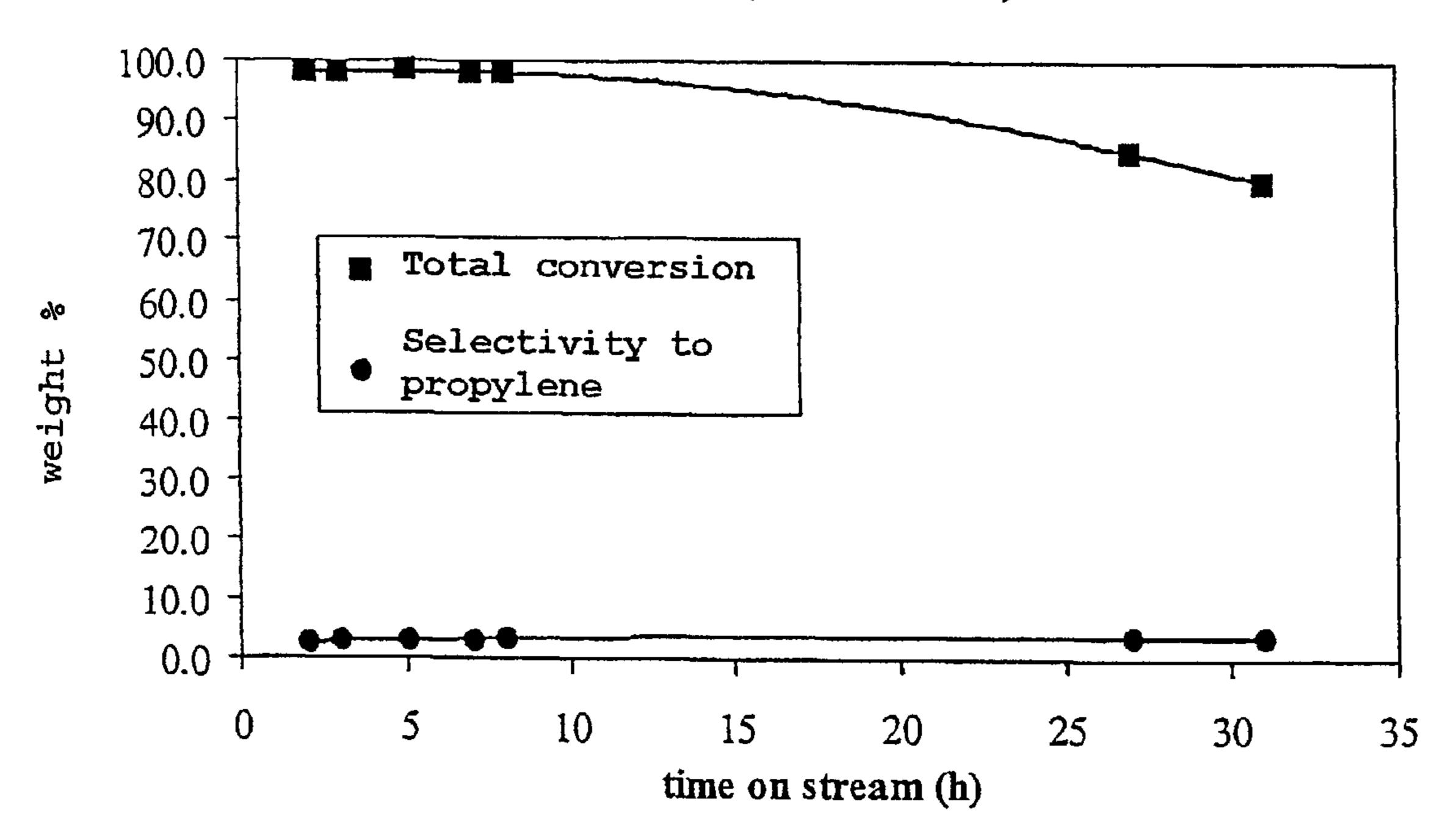
Curves relating to total conversion and selectivity to propylene, obtained with the commercial catalyst ZSM-5 (CBV 3020 E) in relation to the time on stream (h)
