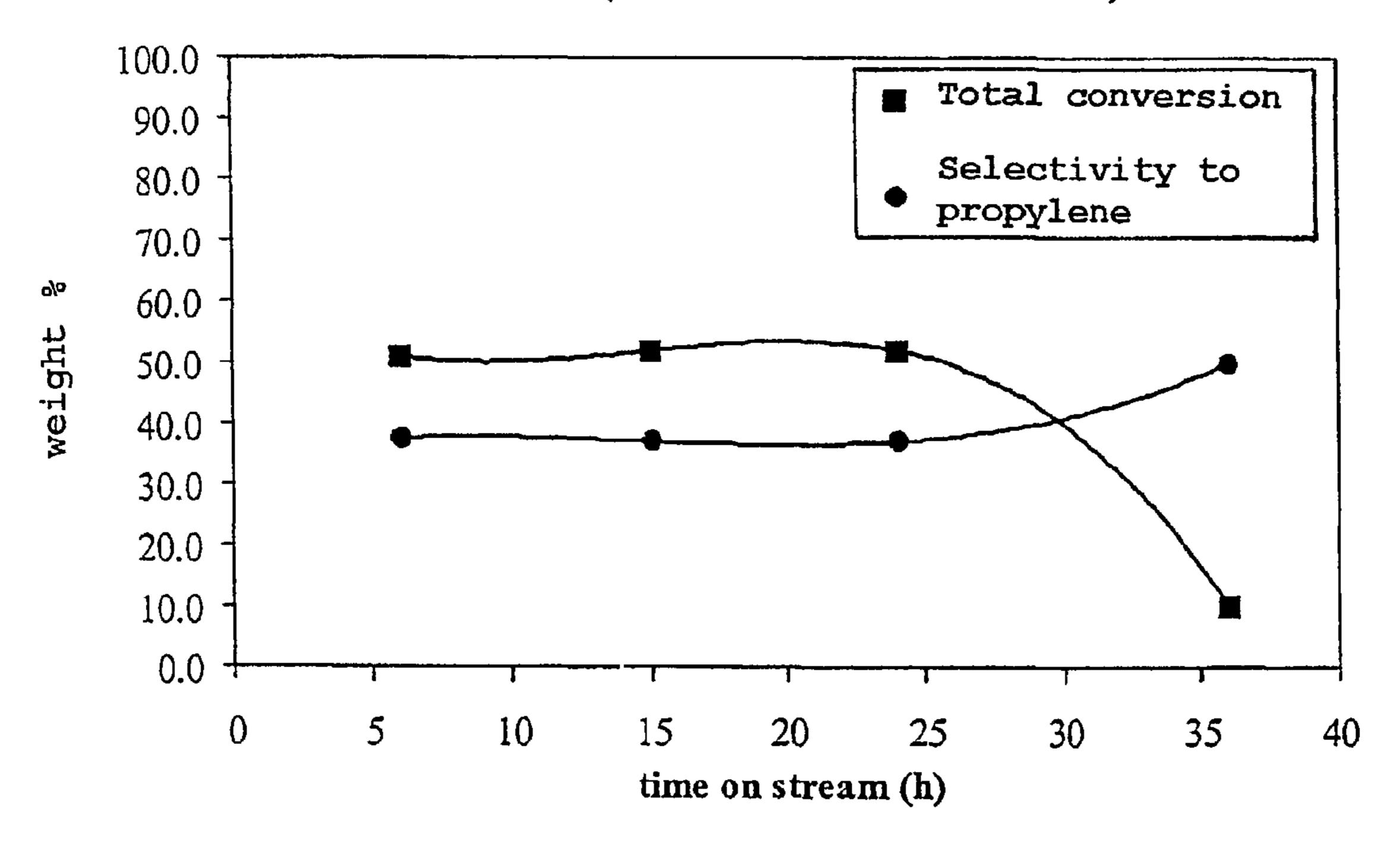
Curves relating to total conversion and selectivity to propylene, obtained with the catalyst ZSM-12 having a molar ratio  $Sio_2/Al_2O_3 = 250$  in relation to the time on stream (h)
