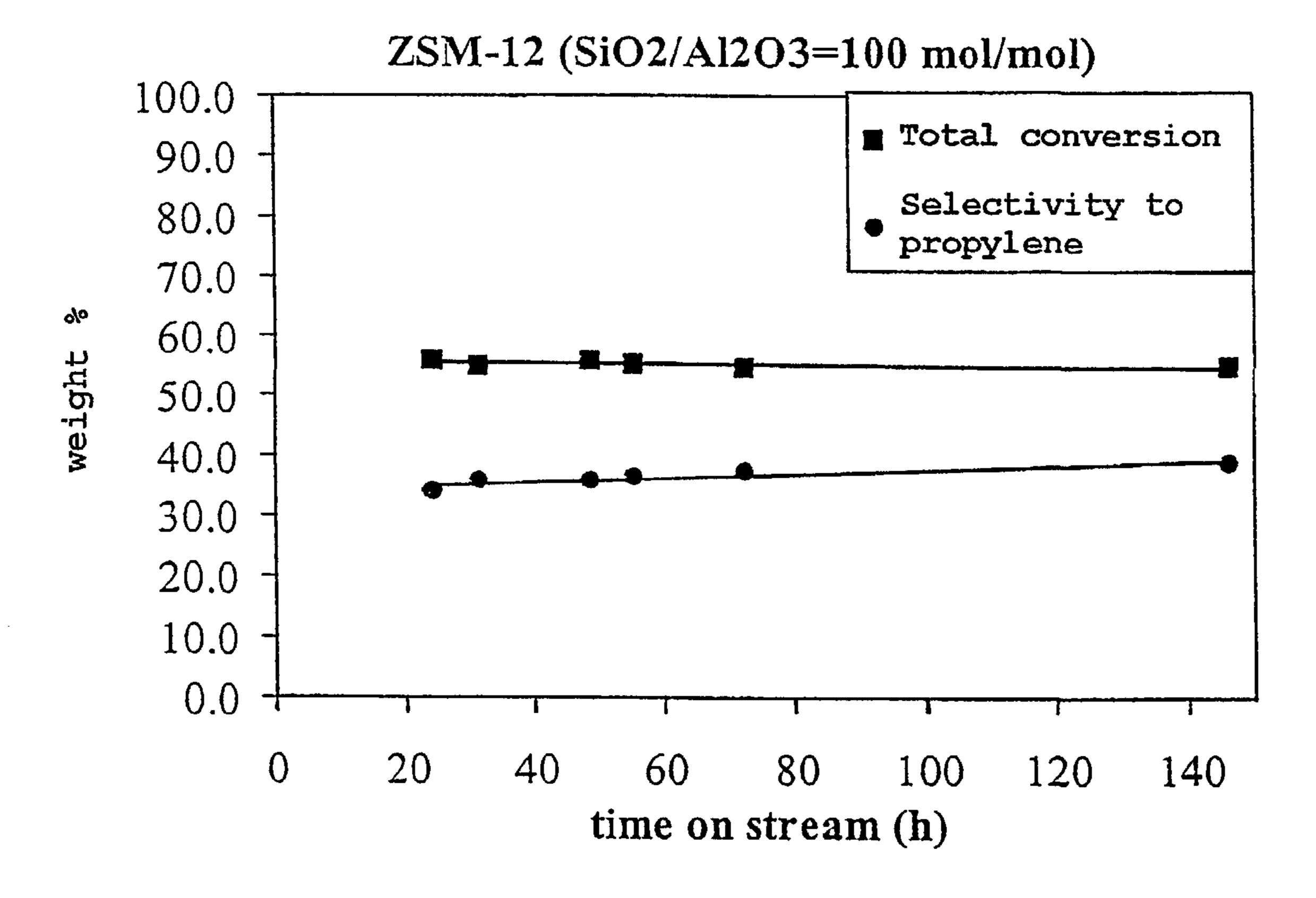
Curves relating to total conversion and selectivity to propylene, obtained with the catalyst ZSM-12 having a molar ratio  $Sio_2/Al_2O_3=100$  in relation to the time on stream (h)
