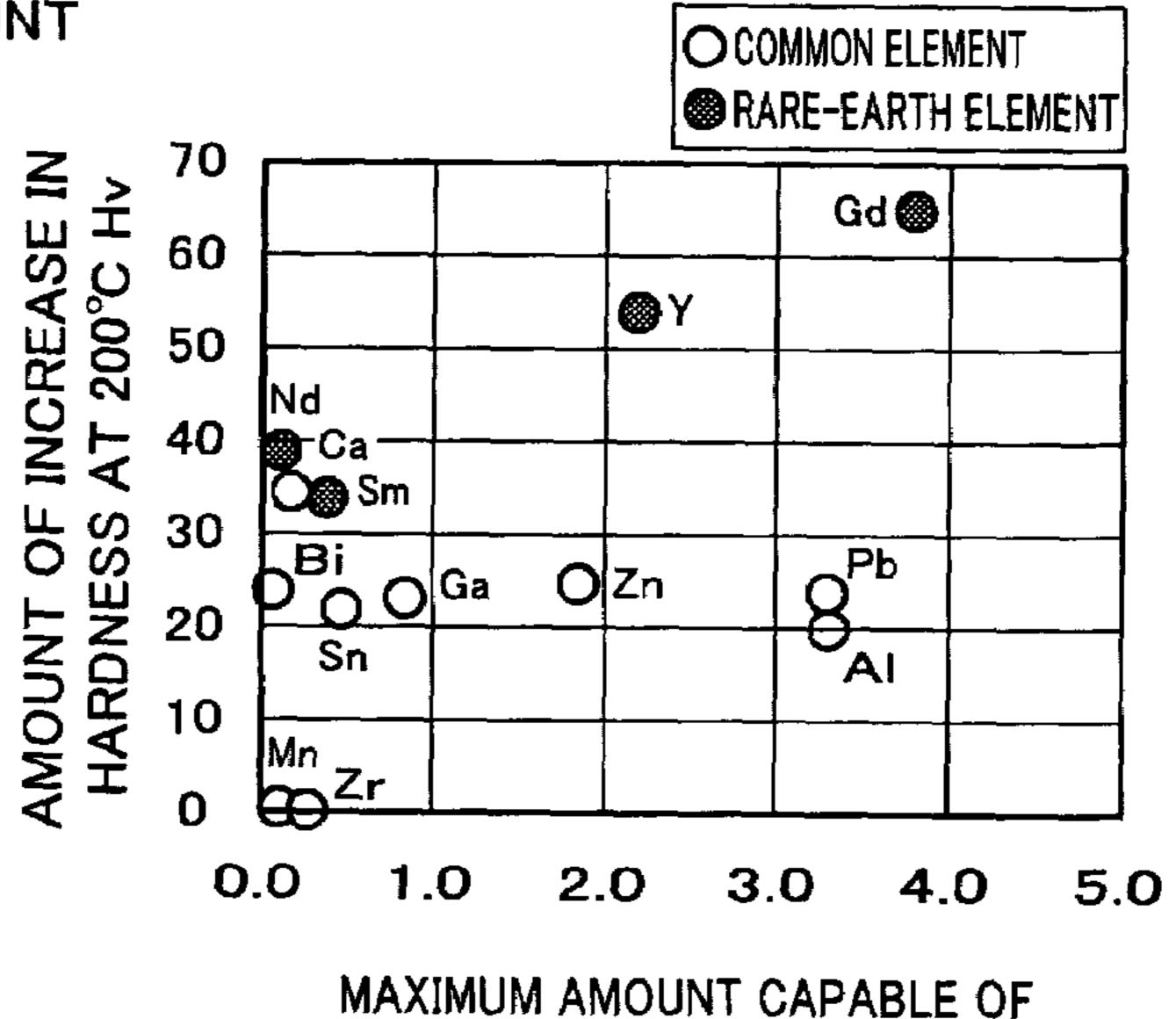
MAXIMUM AMOUNT CAPABLE OF BEING MIXED IN SOLID SOLUTION mass%
