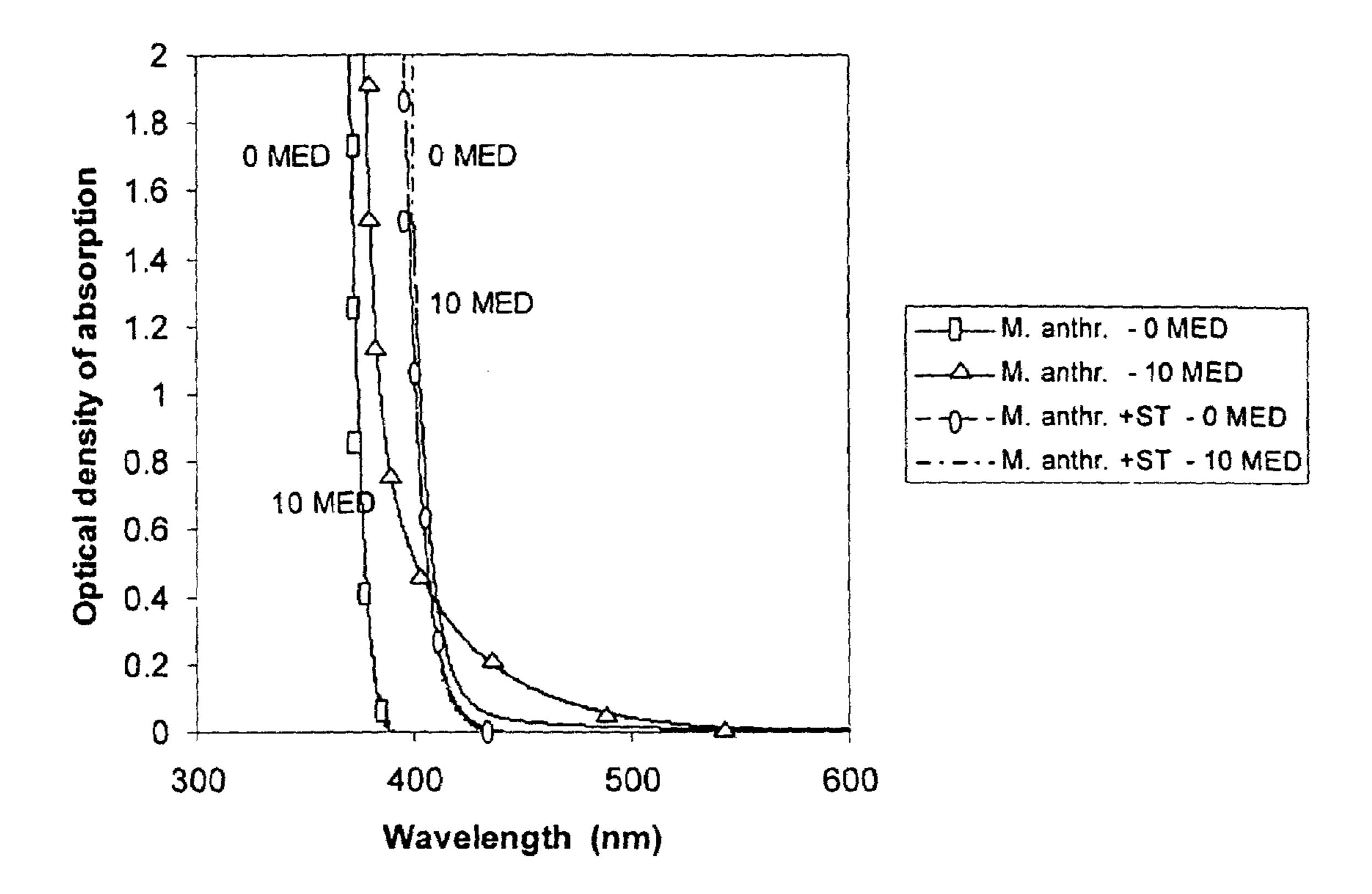
Figure 2: Color change of Menthyl anthranilate (M. anthr.) under sun simulator with and without Diethyhexyl syringylidene malonate (ST) in solution. (Dosage in MED)
