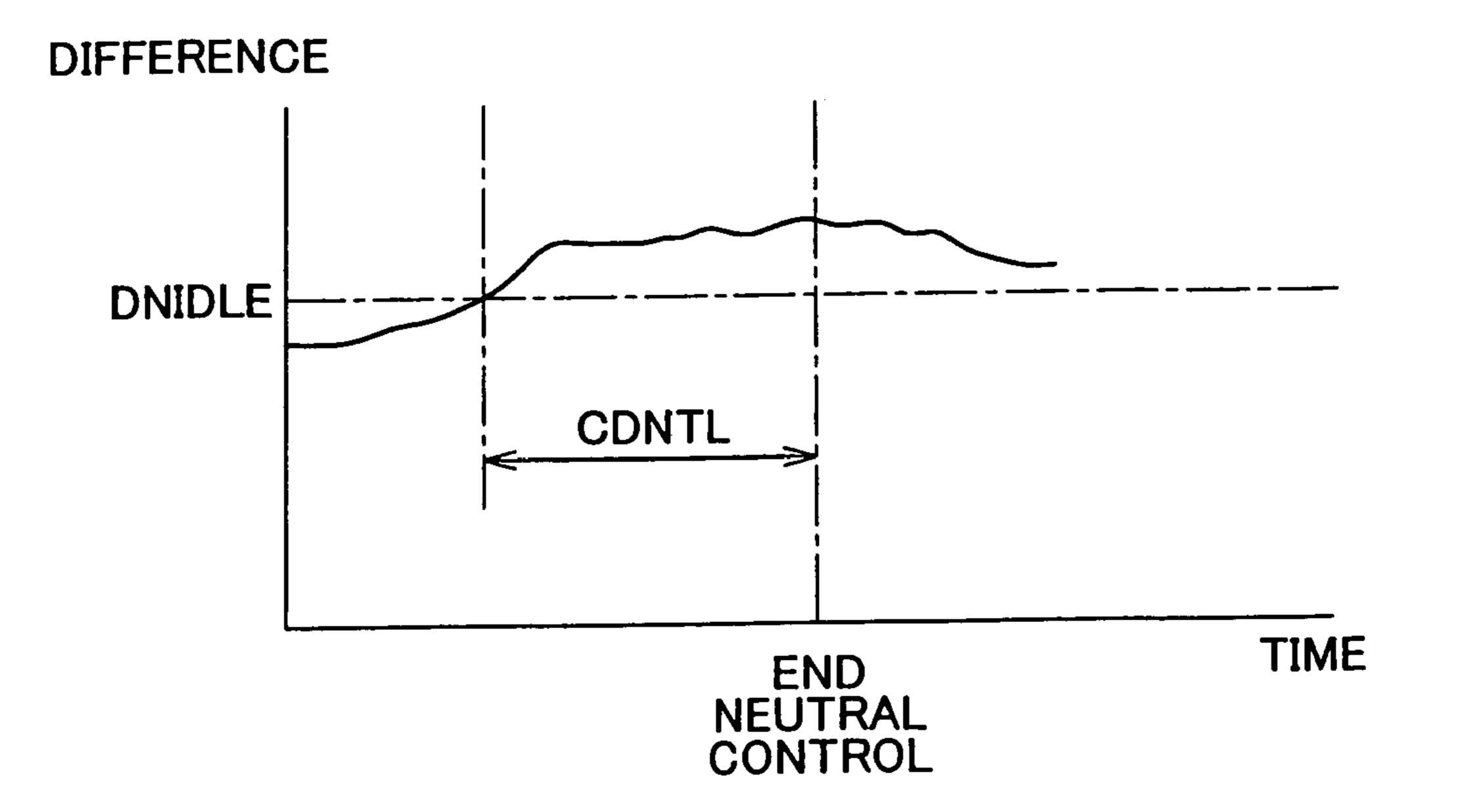
DIFFERENCE = | TURBINE SPEED - TARGET TURBINE SPEED |
