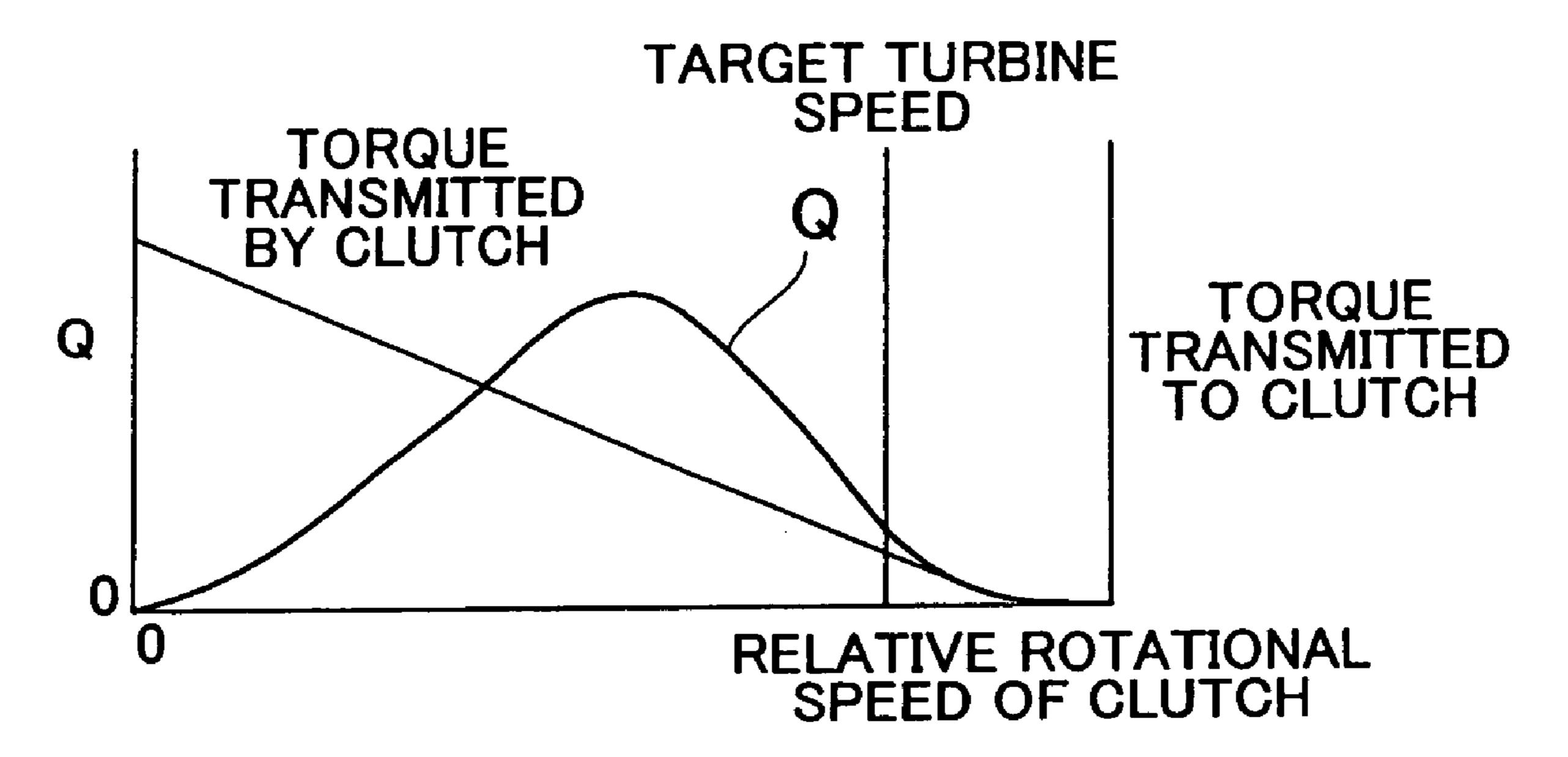
AMOUNT OF HEAT GENERATED INCREASES WHEN TURBINE SPEED DECREASES DUE TO NEUTRAL CONTROL BEING EXECUTED AT TARGET TURBINE SPEED
