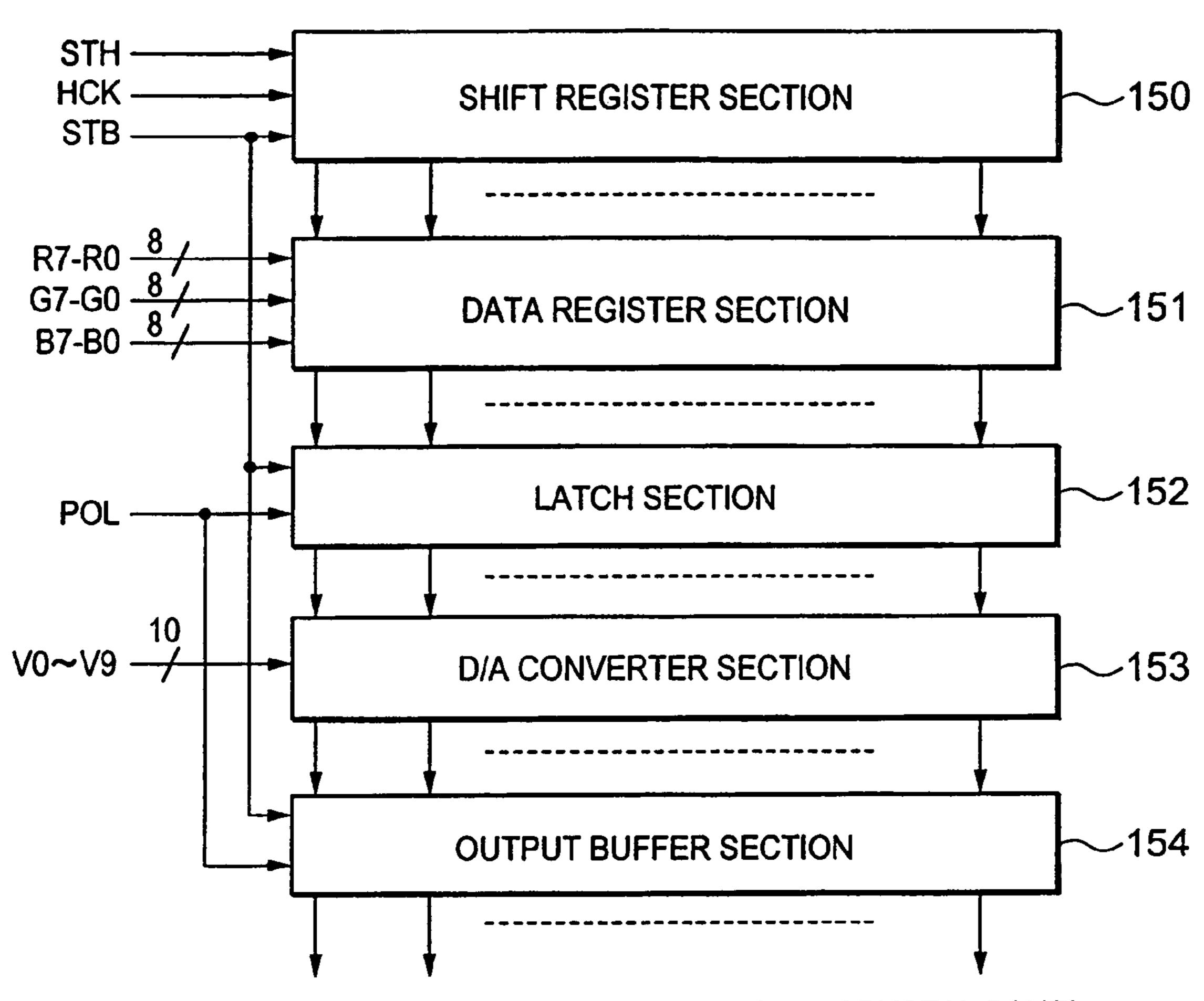
TO INDIVIDUAL SIGNAL LINES OF LIQUID-CRYSTAL PANEL
