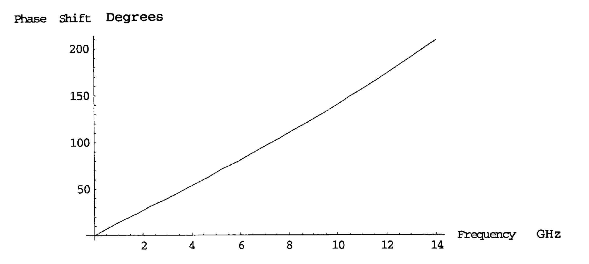
Phase shift vs. frequency for delay line
