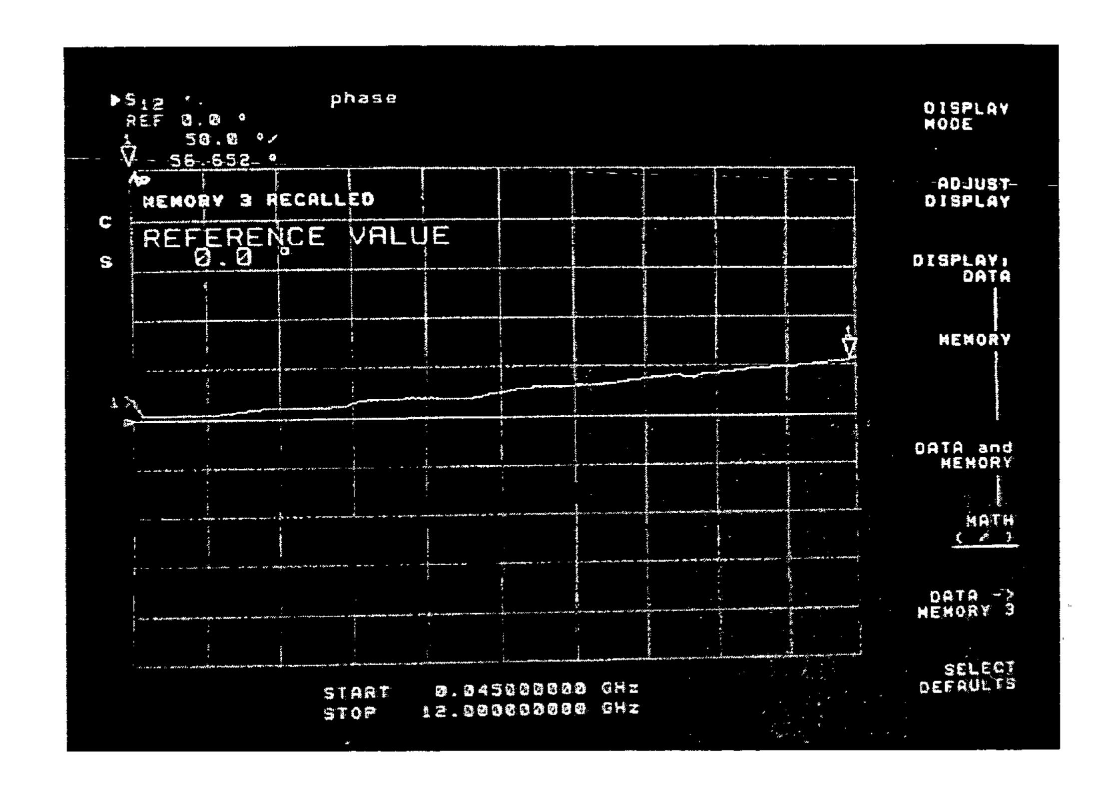
Experimental phase shift vs. frequency for delay line Abscissa: 1 GHz/div, ordinate: 10 degrees/div.
