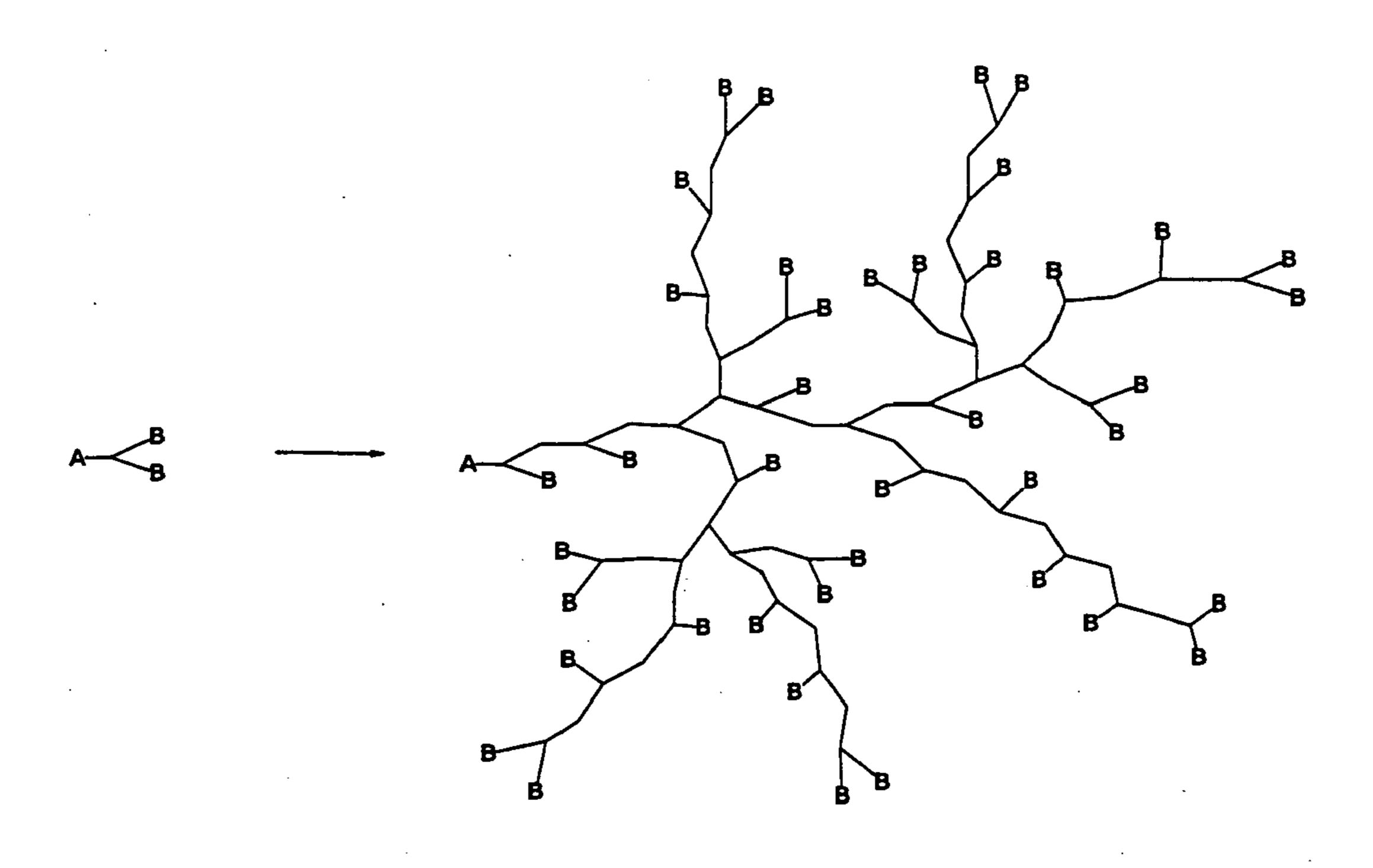
Fig. 1 Schematic synthesis of hyperbranched polymers from  $AB_2$  monomers.
