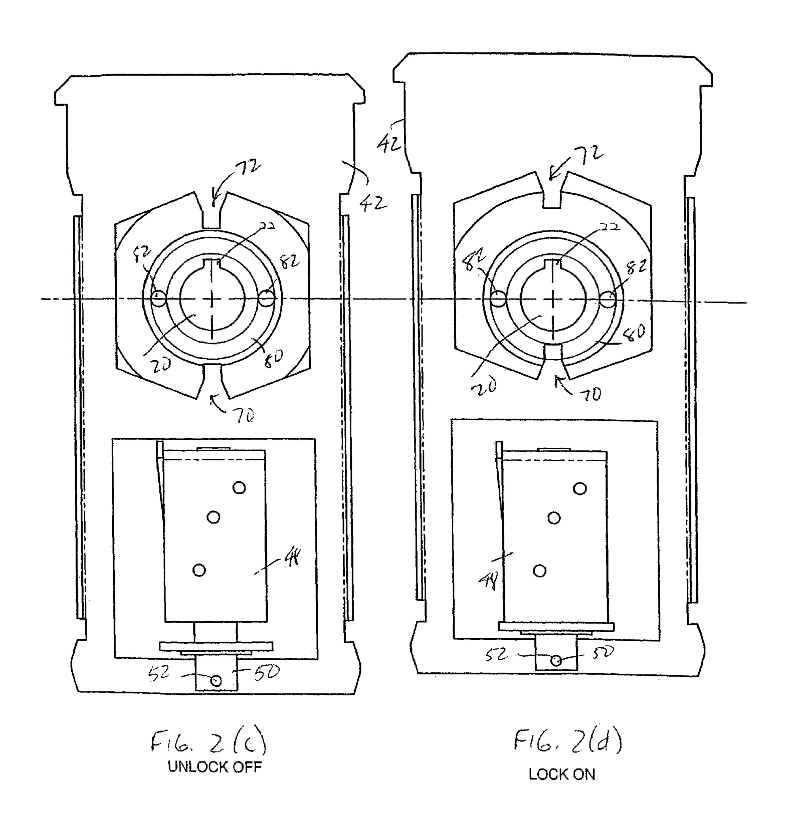
UNLOCKED DURING POWER FAILURE
