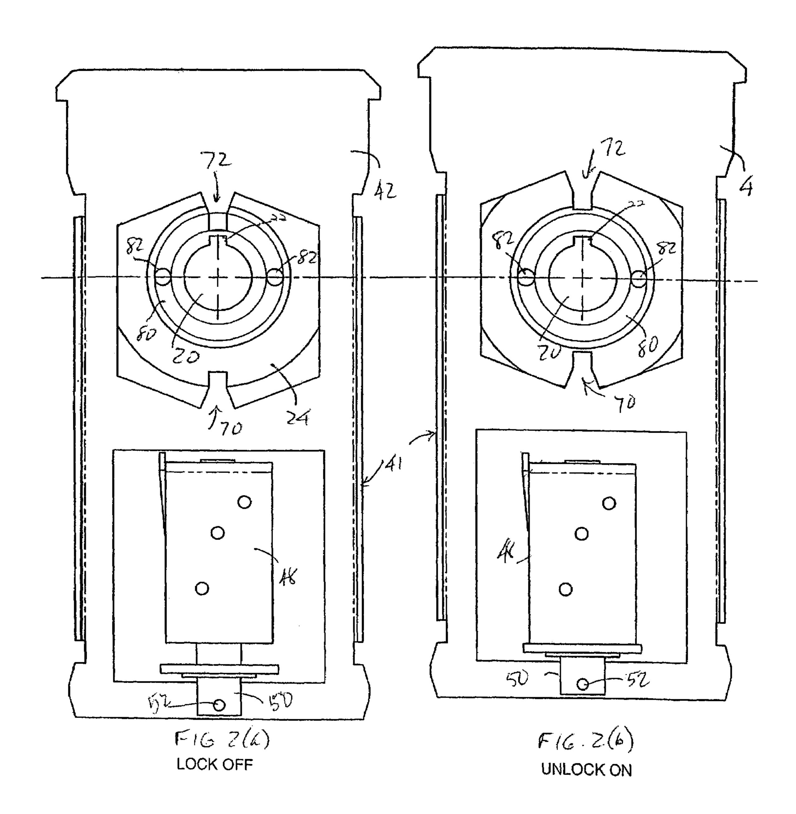
LOCKED DURING POWER FAILURE
