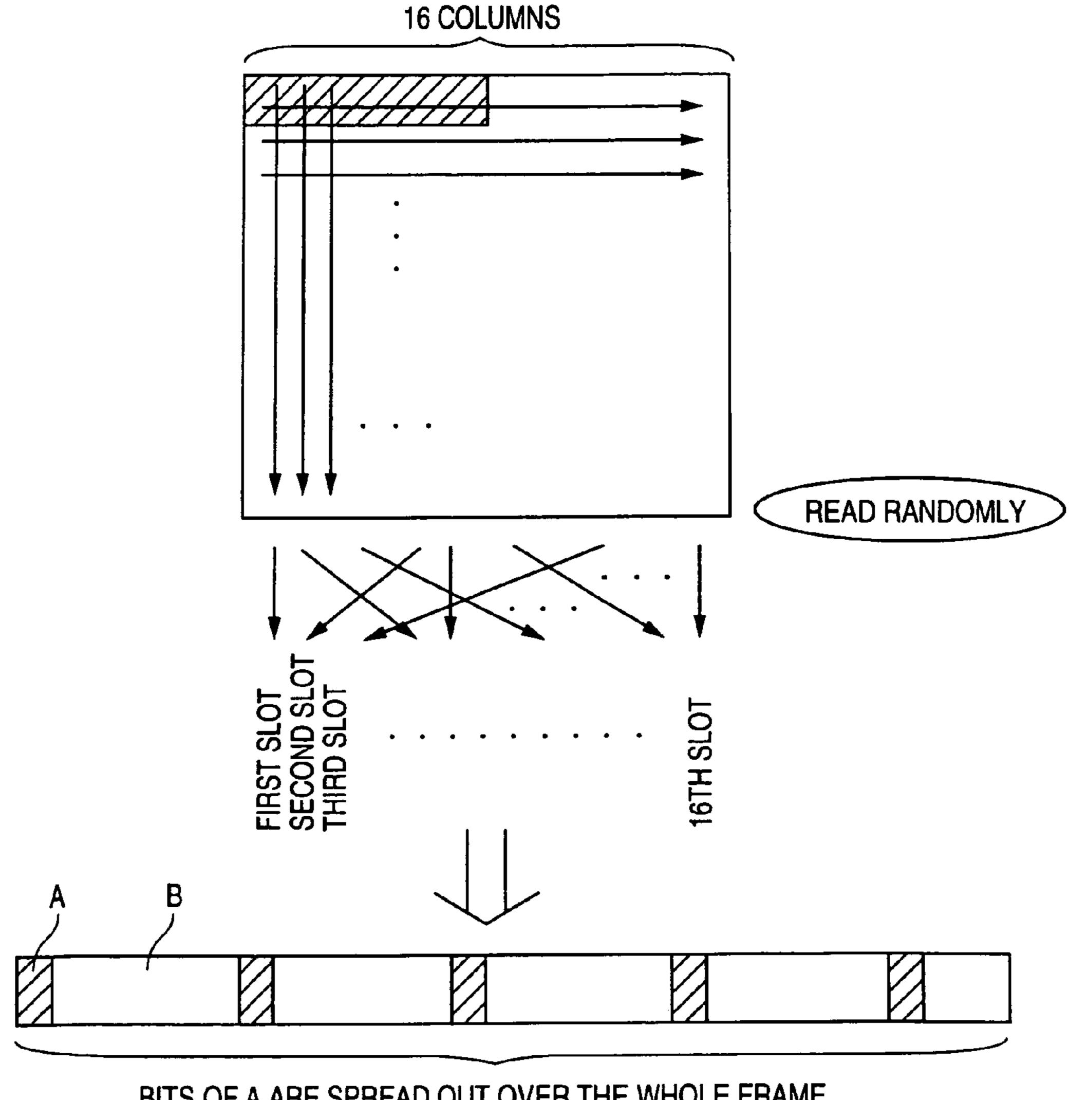
BITS OF A ARE SPREAD OUT OVER THE WHOLE FRAME
