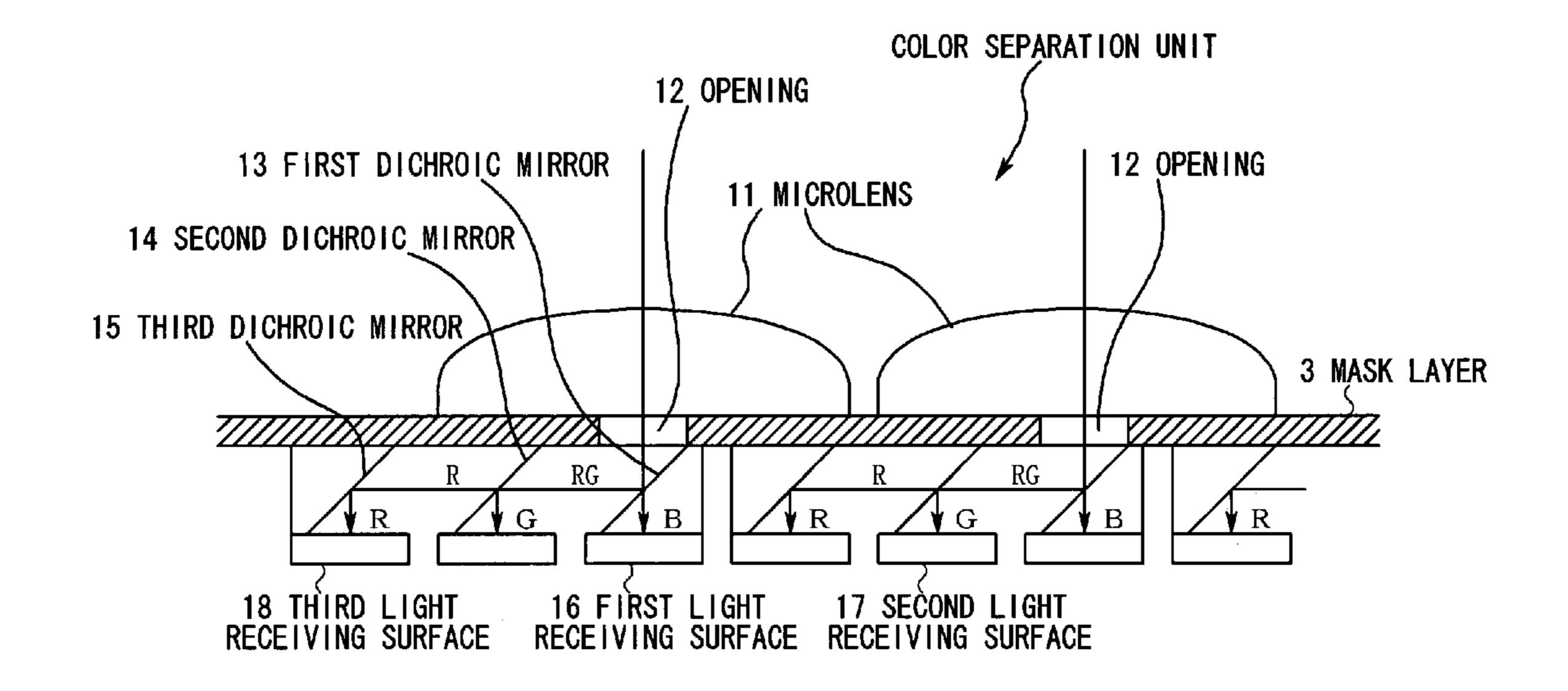
က COLOR SEPARATION MICROLENS MIRROR DICHROIC MIRROR FIRST DICHROLC 15 THIRD DICHROIC MIRROR
