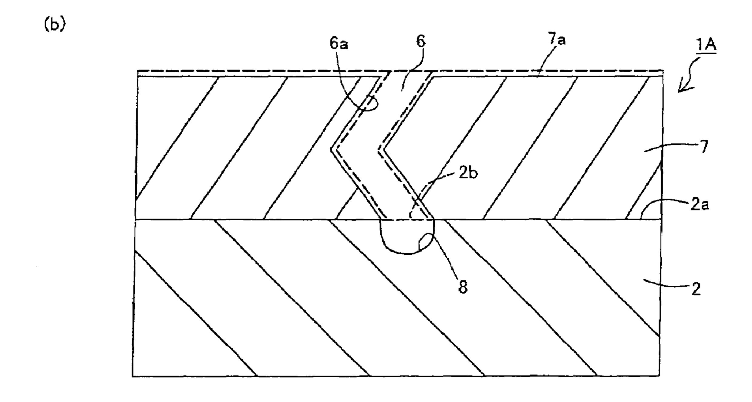
FILM OF YTTRIA-ALUMINA COMPLEX OXIDE, A METHOD OF PRODUCING THE SAME, A SPRAYED FILM, A CORROSION RESISTANT MEMBER, AND A MEMBER EFFECTIVE FOR REDUCING PARTICLE GENERATION
