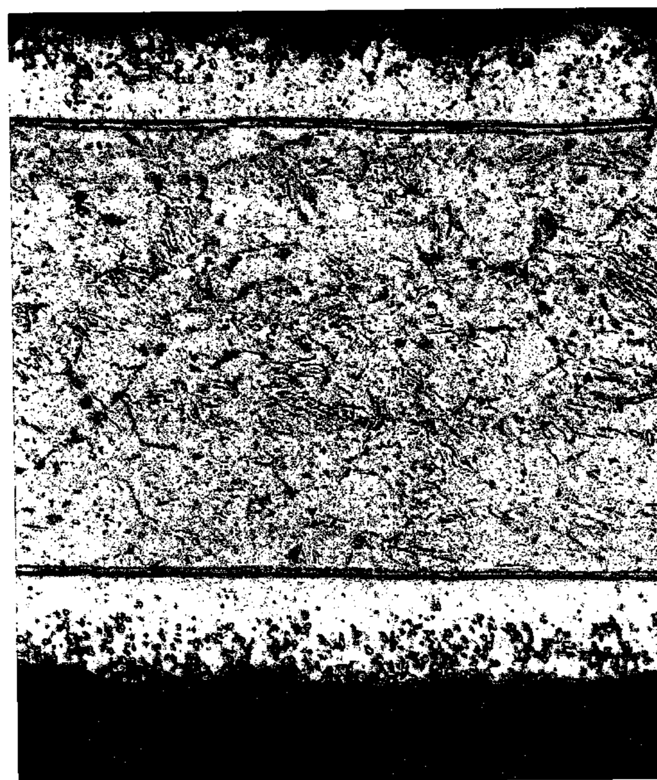
MICROGRAPH OF COATED TITANIUM FOIL AFTER A HEAT TREATMENT BELOW THE MELTING POINT OF ALUMINUM
