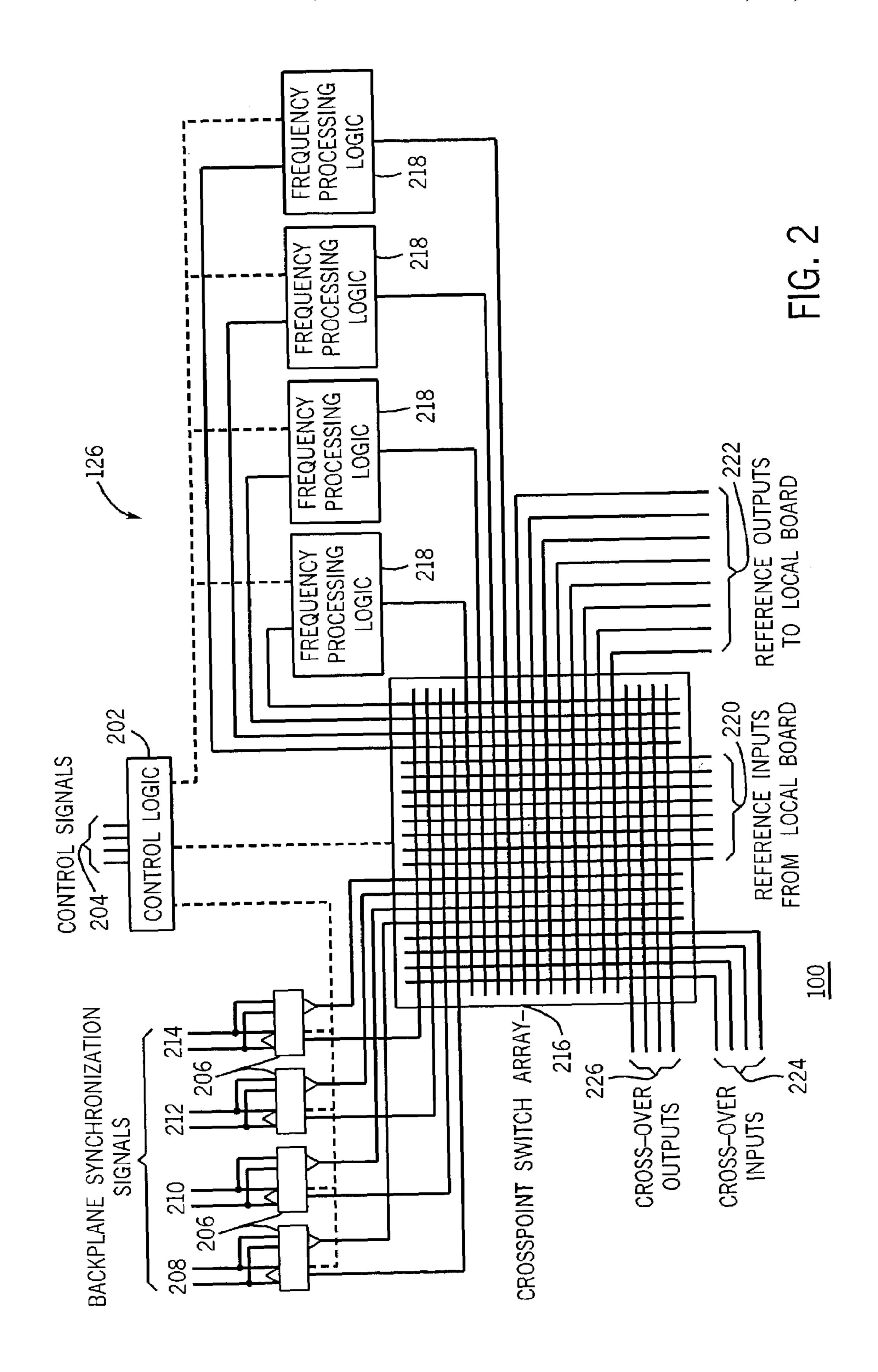
PROGRAMMABLE CLOCK MANAGEMENT COMPONENT RECONFIGURATION UPON RECEIPT OF ONE OR MORE CONTROL SIGNALS TO BE ABLE TO PROCESS ONE OR MORE FREQUENCY SIGNALS
