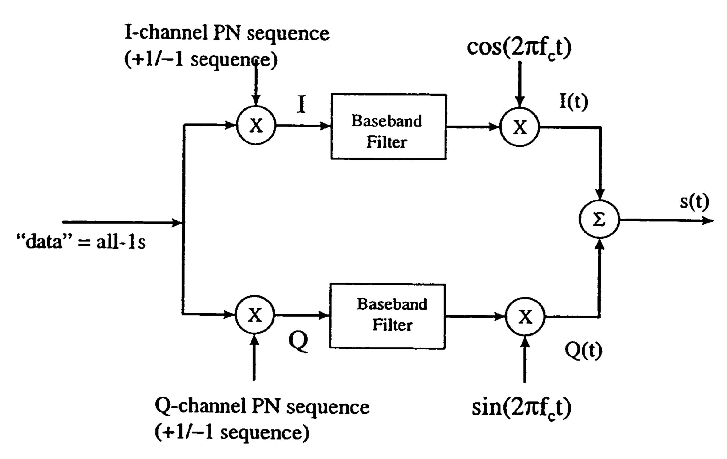
PN'sequence rate = 1.2288 Mcps; period =  $2^{15}$  chips RF carrier frequency =  $f_c$  (Hz)
