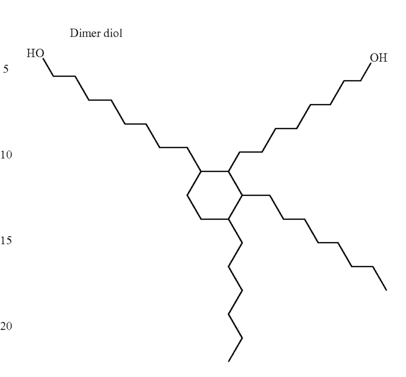
The diol having a cyclic structure and an alkyl chain with two or more carbon atoms is desirably incorporated into the polyurethane resin in a proportion of 5 to 60 mass percent, preferably 10 to 40 mass percent. When the content of diol having a cyclic structure and an alkyl chain with two or more carbon atoms is within the stated range, solubility in solvent is high, good dispersibility is achieved, and durability is good.
