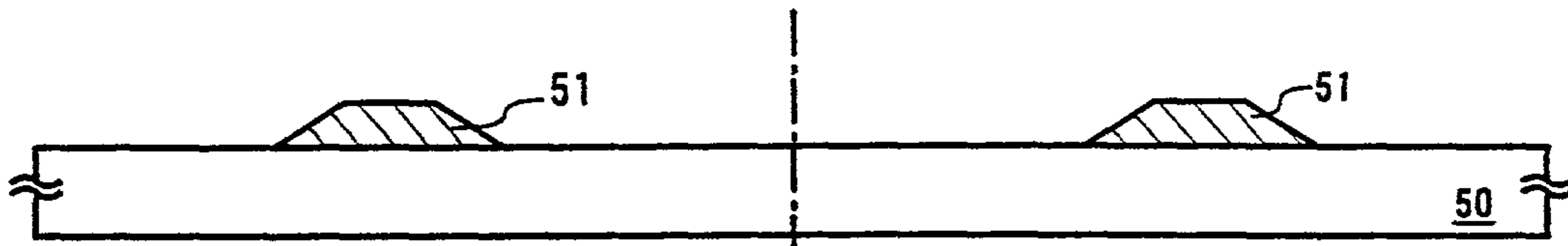
FIG. 8(b) FORMATION OF GATE INSULATING FILM AND SEMICONDUCTOR FILM
