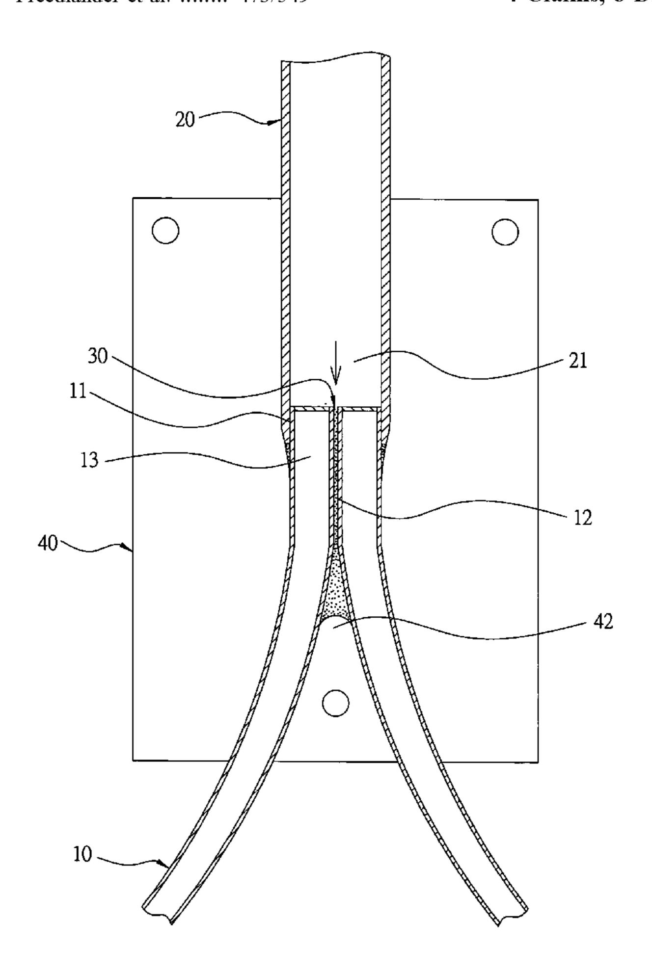
Preparing a metal racket frame, a hollow grip, a proper amount of liquid resin and a matched mold.
