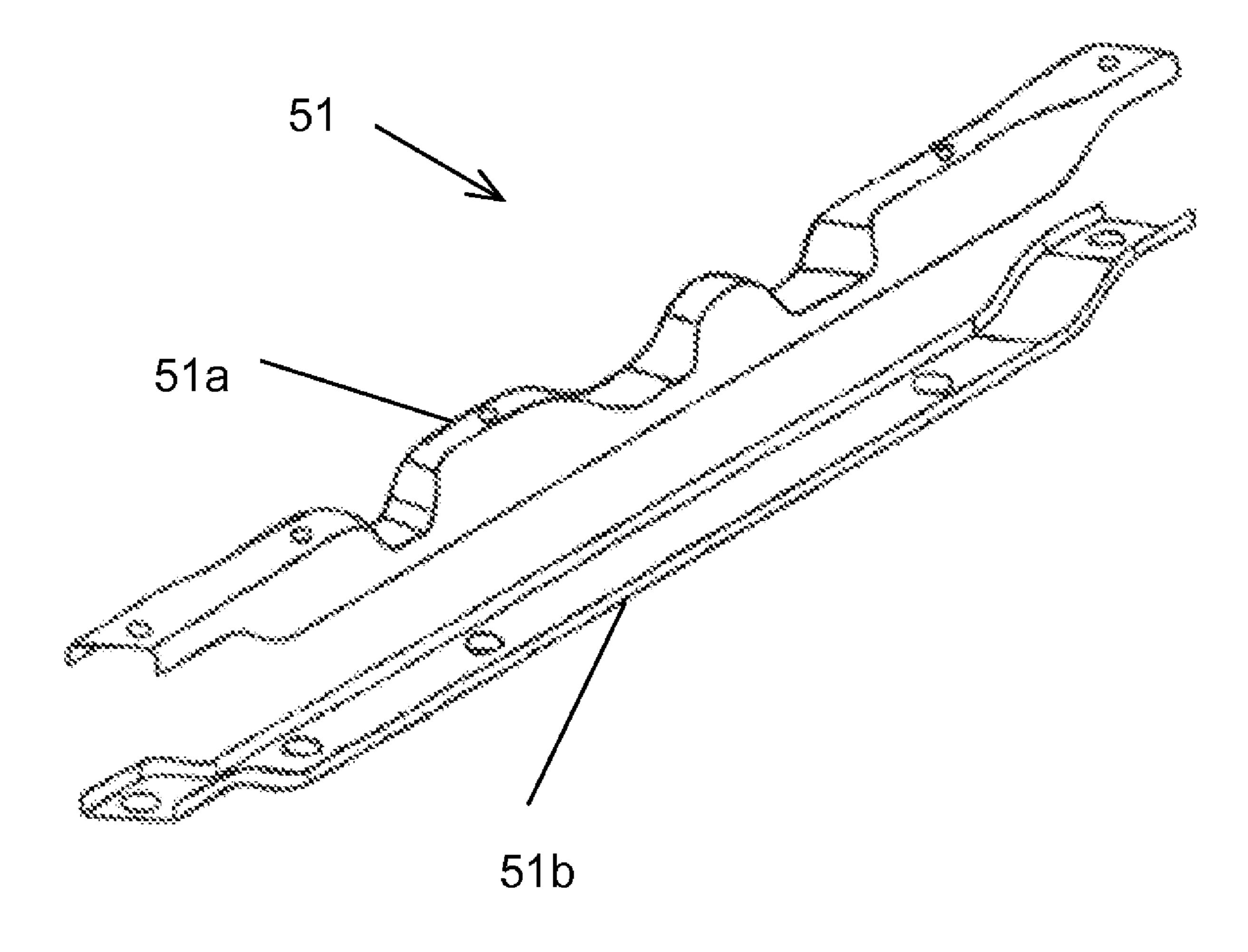
The present invention relates to a motor vehicle chassis comprising two lateral longitudinal members between which extend transversely and to which are affixed the front floor part, the rear floor part, a cross member called "heel board" cross member whose upper and lower longitudinal sides are
