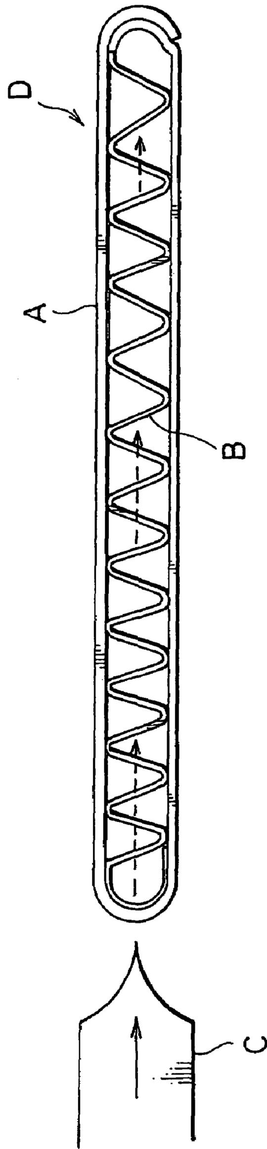
**TUBE FOR HEAT EXCHANGER**
