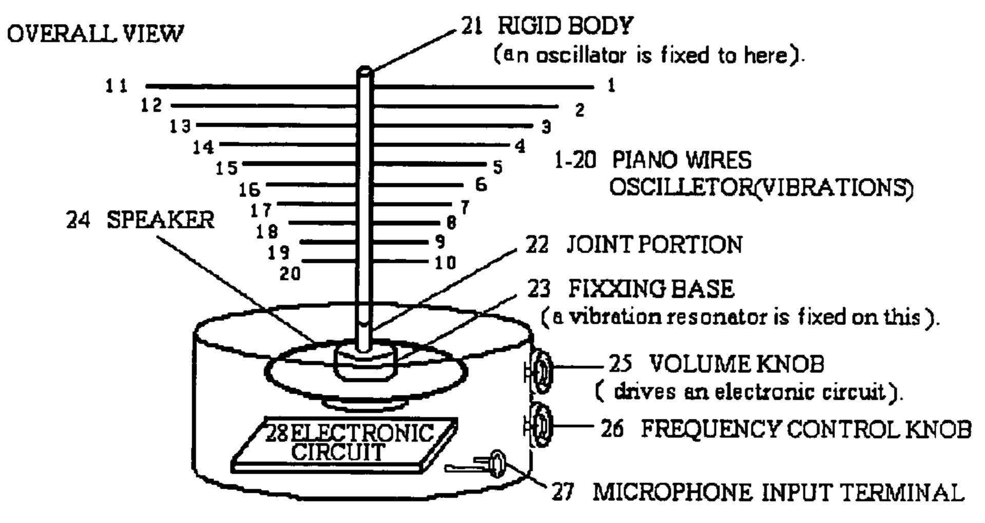
SOUND/VIBRATION RESONANCE SEPARATING DEVICE
