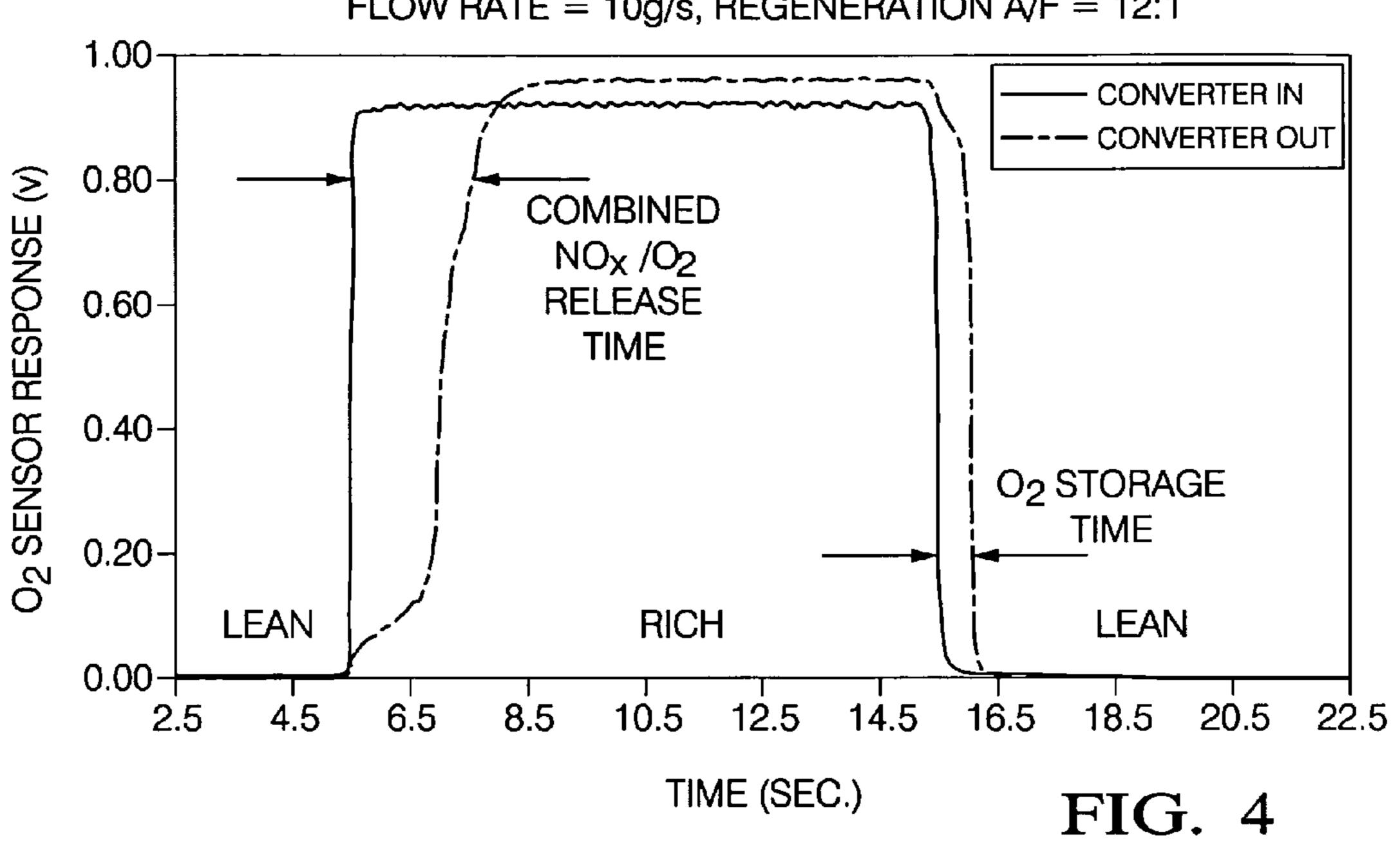
1.7L NO<sub>X</sub> ADSORBER, AGED 10 HRS AT  $400^{\circ}$ C, EVAL AT  $480^{\circ}$ C FLOW RATE = 10 g/s, REGENERATION A/F = 12:1
