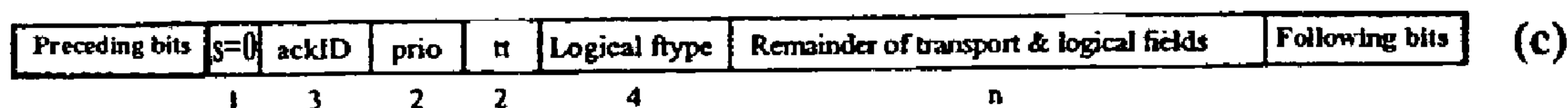
Flow Control Fields Bit Stream
