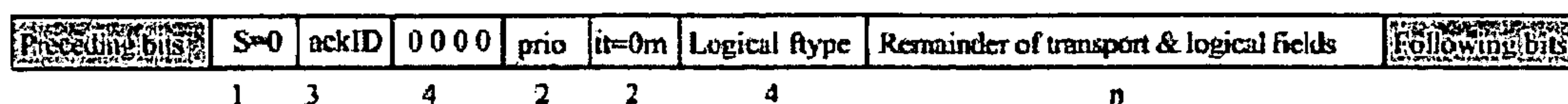
Figure 7. Packet Bit Stream
