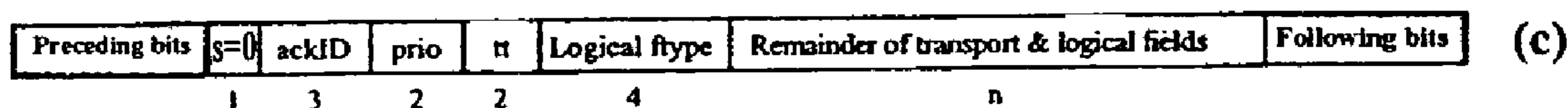
Flow Control Fields Bit Stream
