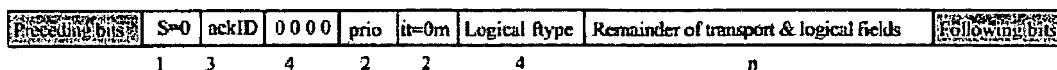
Figure 7. Packet Bit Stream
