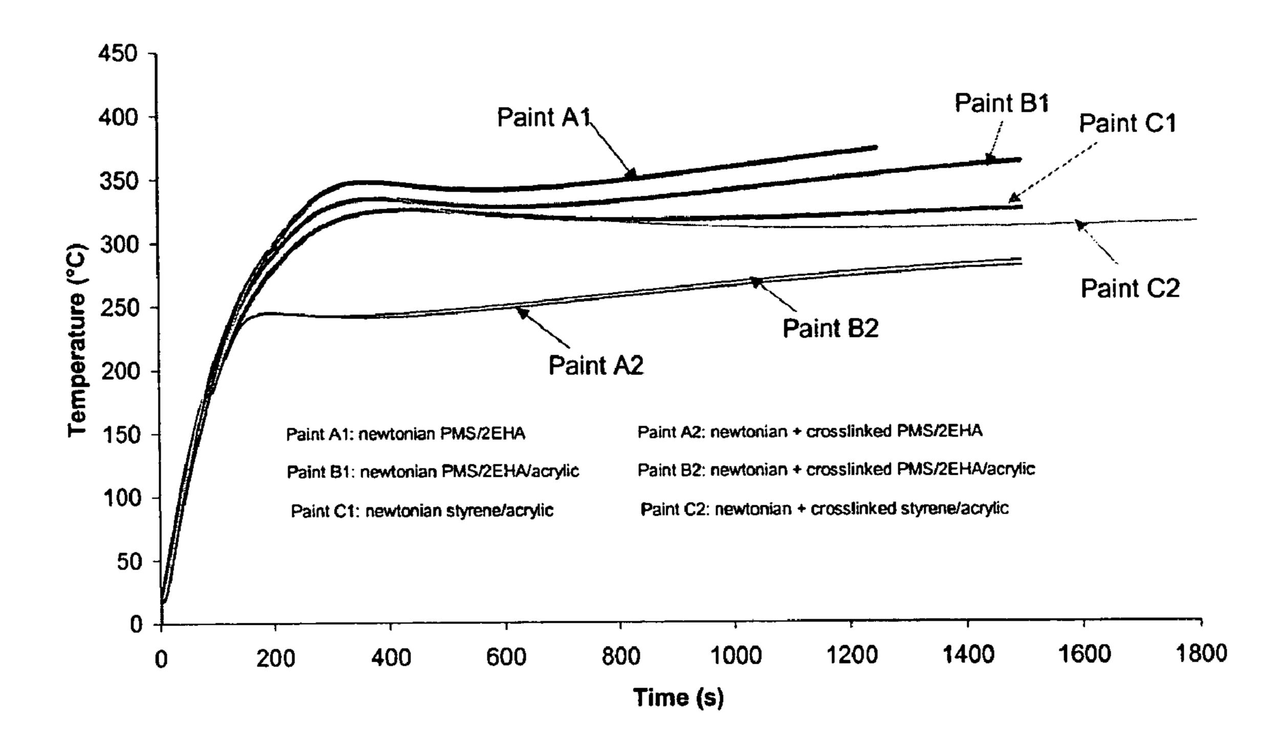
Thermal insulation on aluminium plates with intumescent coatings prepared with PMS/2EHA and with styrene/acrylic resins
