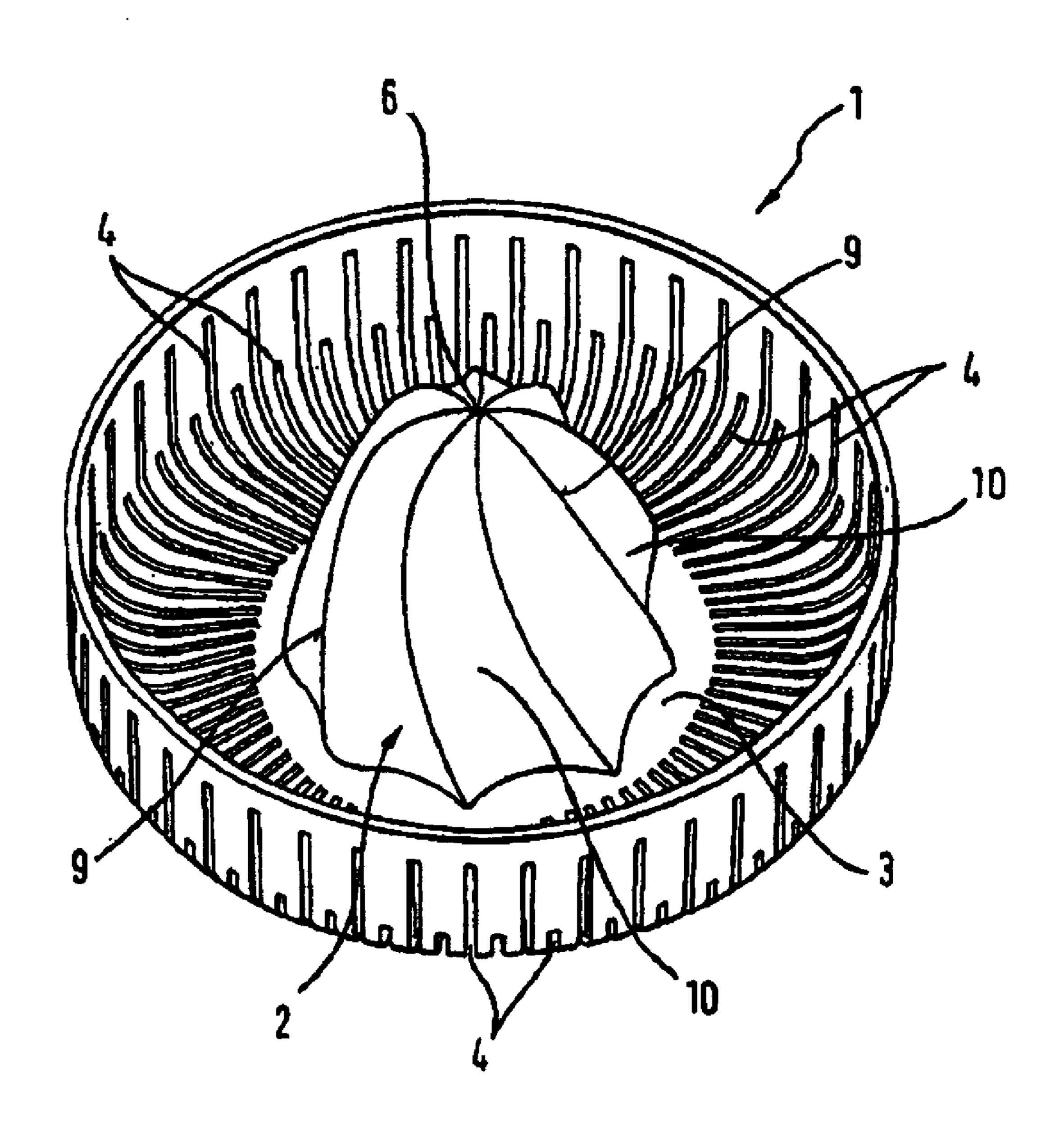
The present invention relates to a fruit press comprising a centrally arranged, projecting element which tapers to the top for the pressing of a fruit and an annular surface surrounding the base of said element, whereby the element has ridges on its outer surface, running from the base of the element upwards, between which trough-shaped recesses are arranged.
