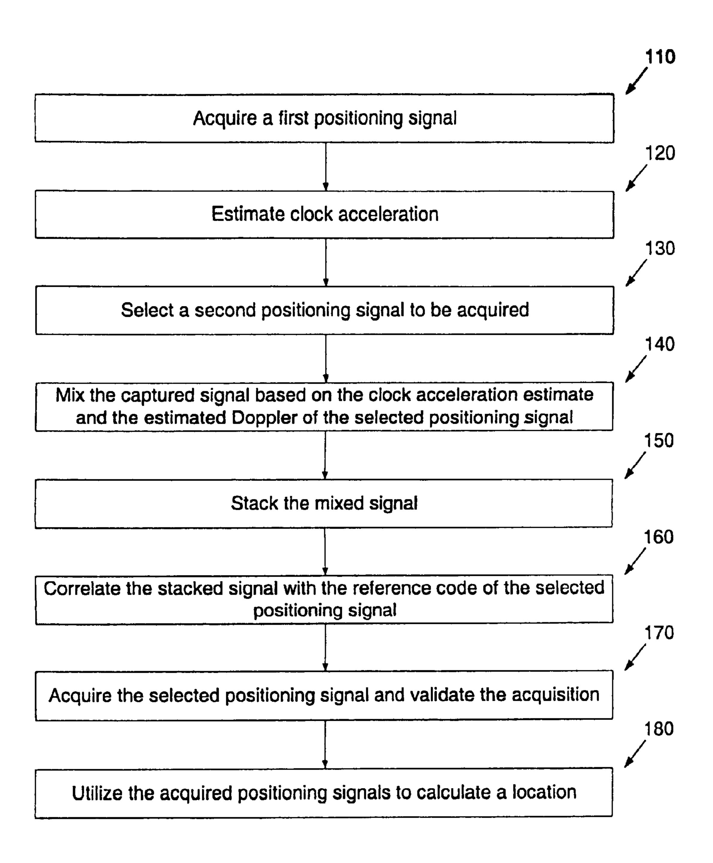
Fig. 1. Method for acquiring positioning signals and calculating a location
