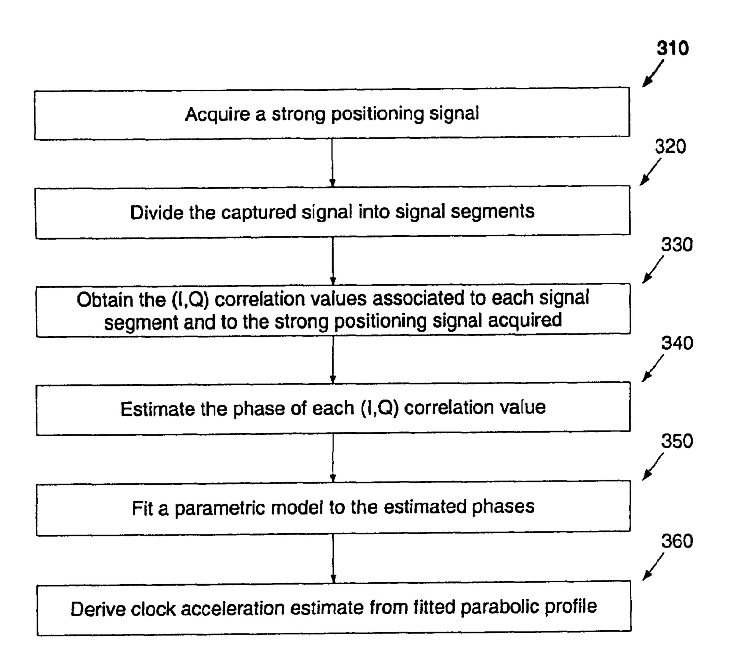
Fig. 3. Method for estimating clock acceleration
