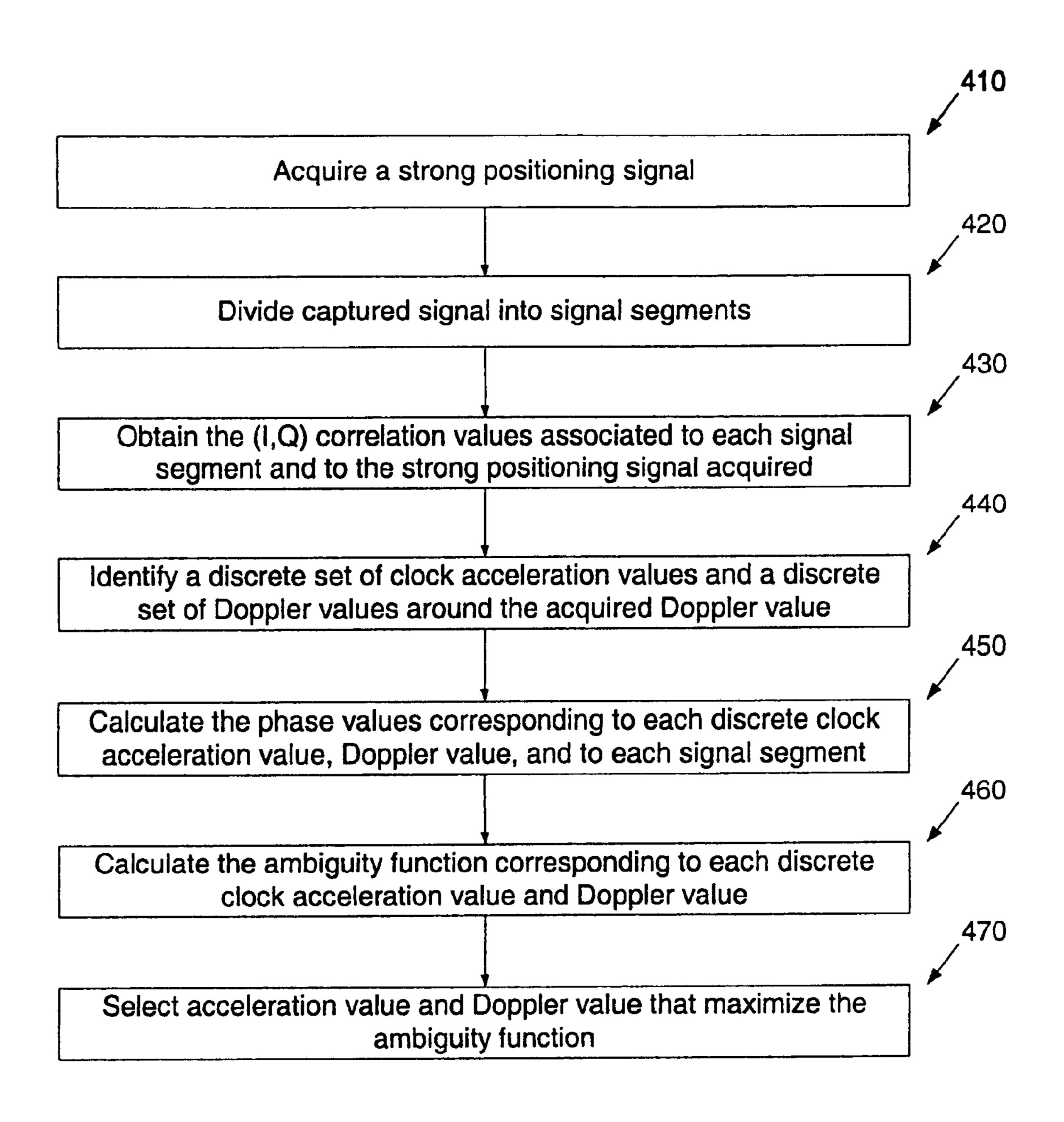
Fig. 4. Method for estimating clock acceleration
